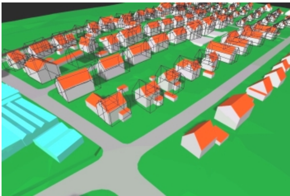
Figure 4: Practical application example of a 3D study: Intersection of buildings and planned construction boundaries.
