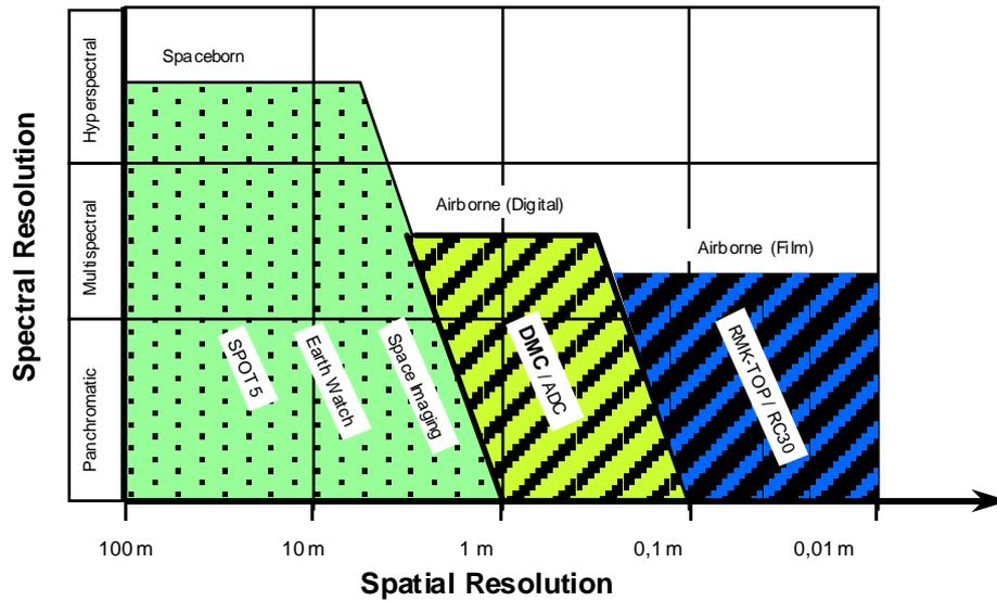
Figure 5: Positioning of Sensorsystems.
