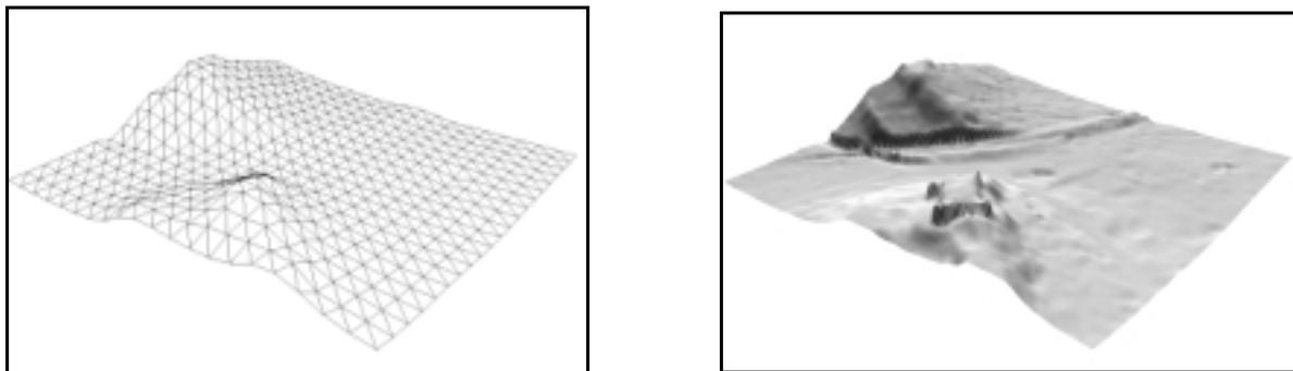
Figure 1: Perspective 3D Views derived from official DTMs.
