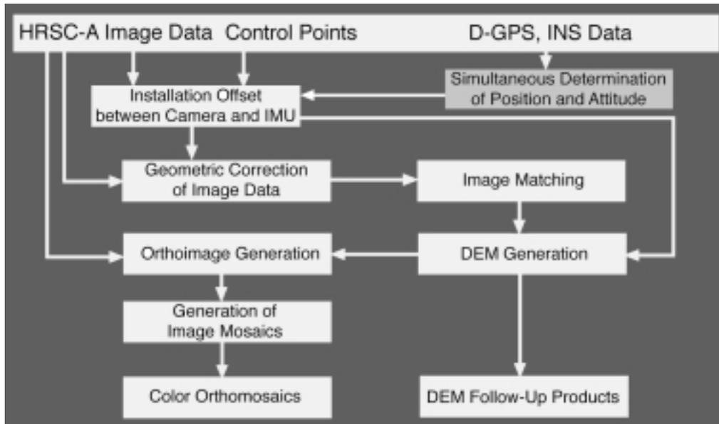
Figure 2: Photogrammetric Processing Line for HRSC-A.
