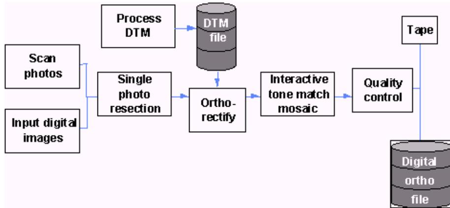
Figure 1: Orthophoto Rectification and Mosaicking Workflow.
