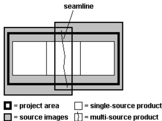
Figure 8: Single-source and Multi-source Ortho Products.
