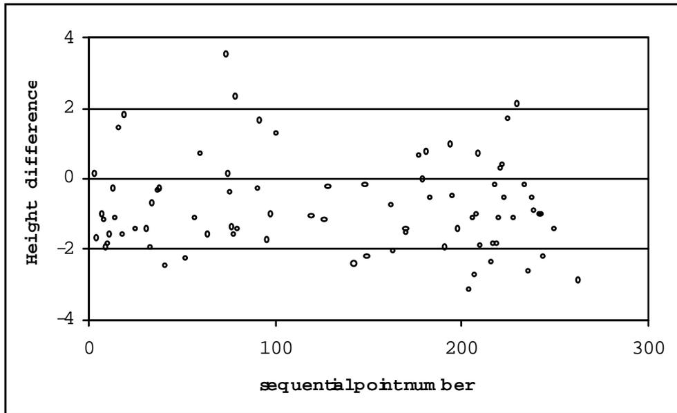
Figure 3: Height differences for 79 Trigonometric Points in open terrain.
