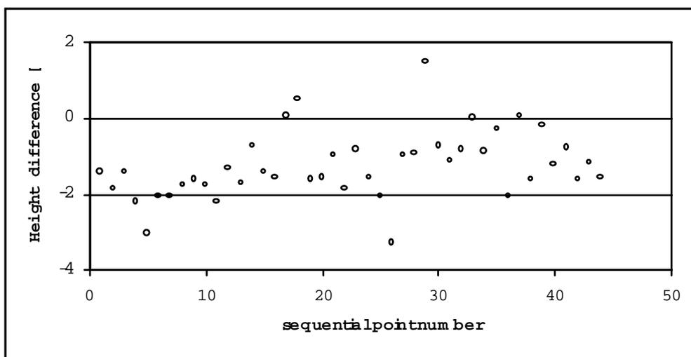
Figure 4: Height differences for 44 reference points determined with GPS.
