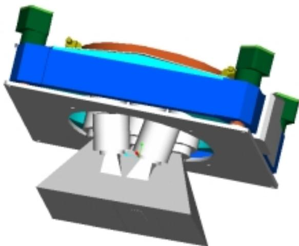
Figure 3: Illustration of optical arrangement of 7 head camera.
