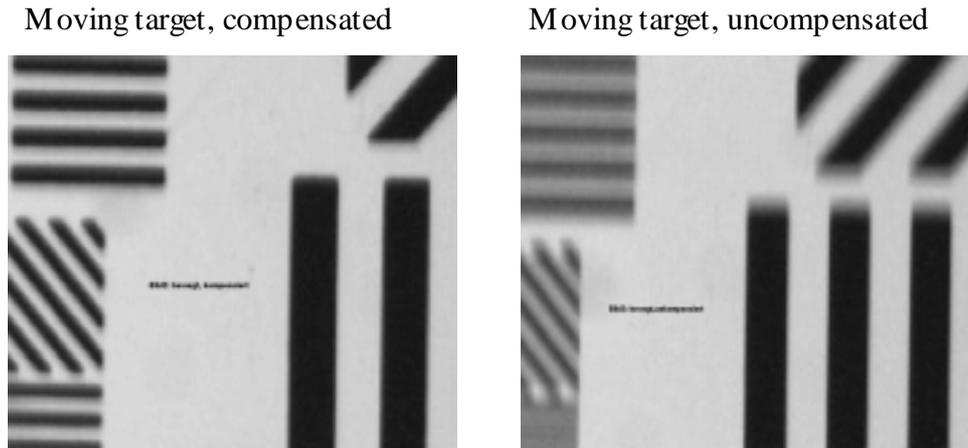
Figure 5: Resolution target with / without motion compensation.
