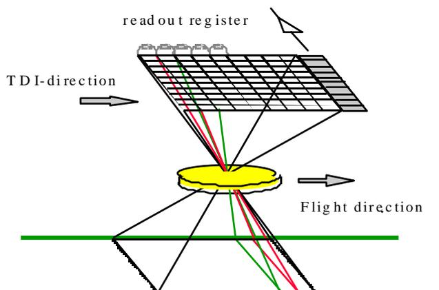
Figure 4: Principle of time delayed integration.
