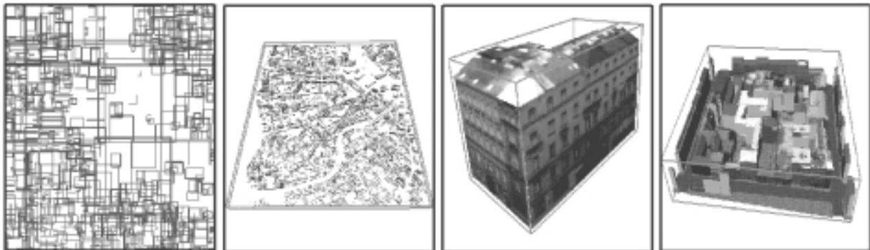
Figure 4: R-tree structure of an entire city and related levels of detail. From left to right: Level 0: Entire city, links to the lower R-tree level, links to the 2D GIS (optional), no CAD data. Level 1: One district, links, low resolution CAD data. Level 2: One city block, links, medium resolution CAD data. Level 3: One Building, links, high resolution CAD data.
