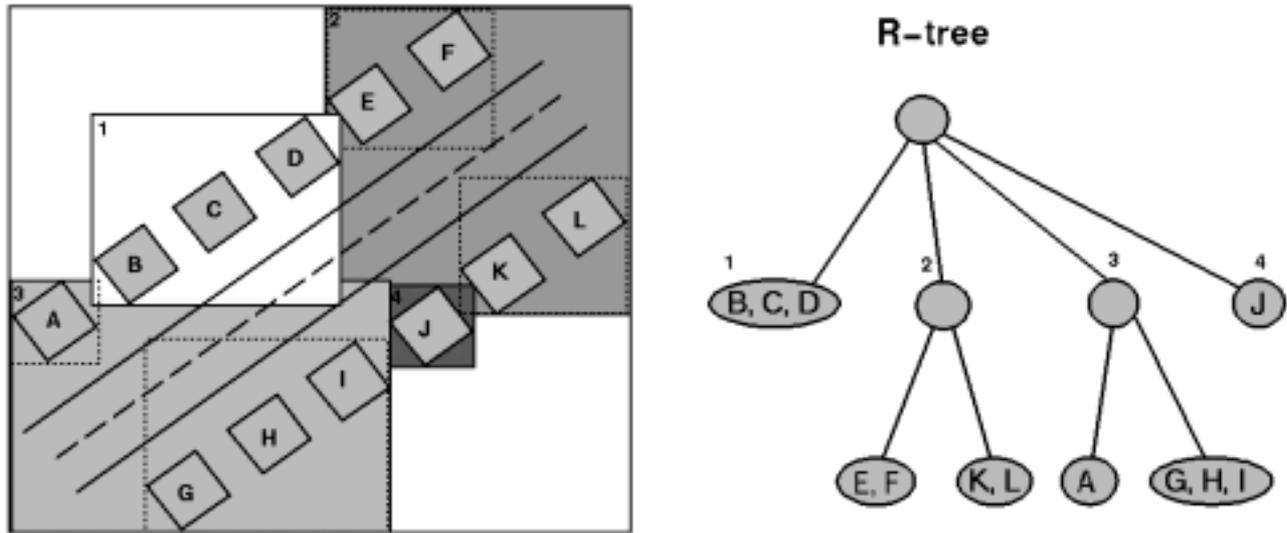
Figure 3: Principal concept of the R-tree data structure. Buildings on both sides of a street are organized by rectangular bounding boxes (left) and the related R-tree (right).
