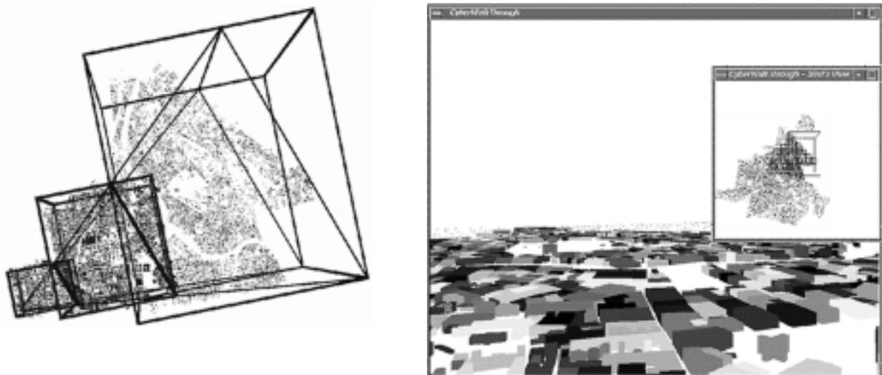
Figure 5: The Vienna walk trough System, as implemented on a Silicon Graphics desktop Workstation. The navigation during interactive visualization (large viewport, right) is supported by a vertical view (small viewport, right). The data loading is organized through a 3D view frustum (left).
