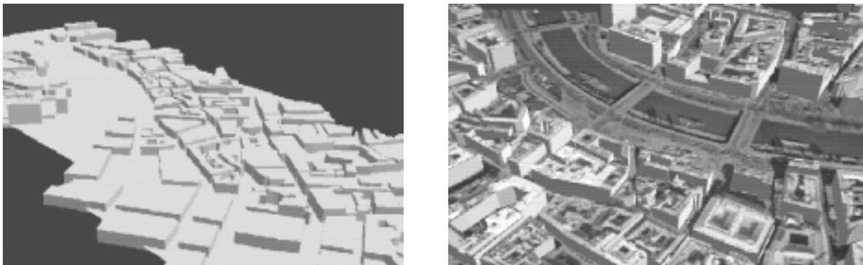
Figure 2: Three dimensional data of a city. Left: Pure geometry data at a course level of detail (building blocks and terrain data); Right: Phototexture from aerial images mapped onto the horizontal surfaces of the model.
