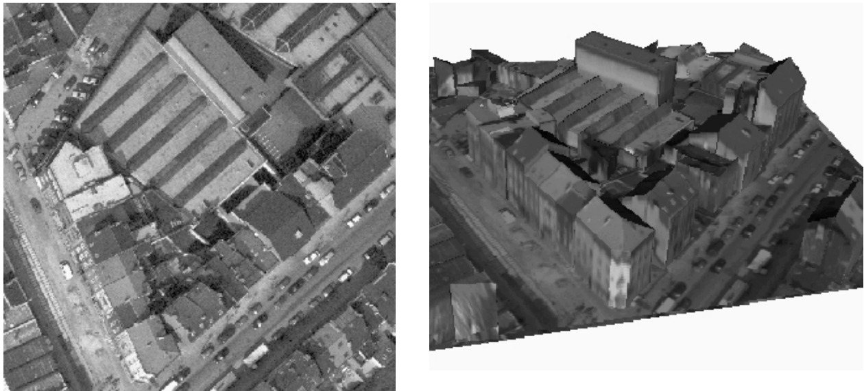
Figure 1: shows one image (section) out of 6 and the automatically derived texture mapped 3D model, from Baillard et al. 1999.
