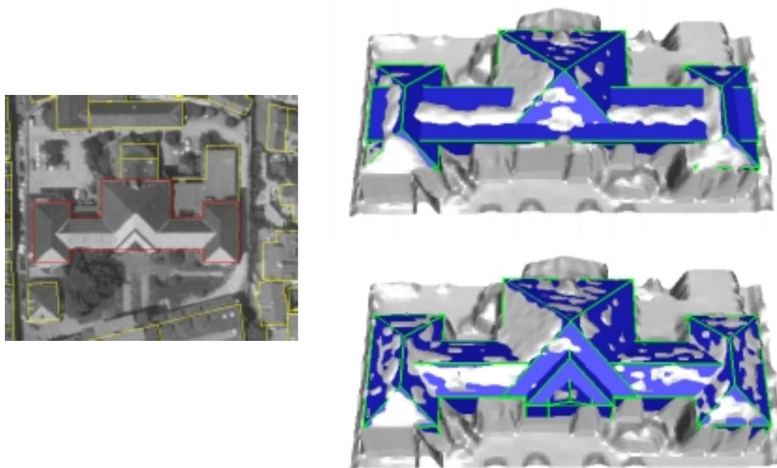
Figure 6: Ortho image (left) and reconstruction before (top) and after (bottom) manual editing.
