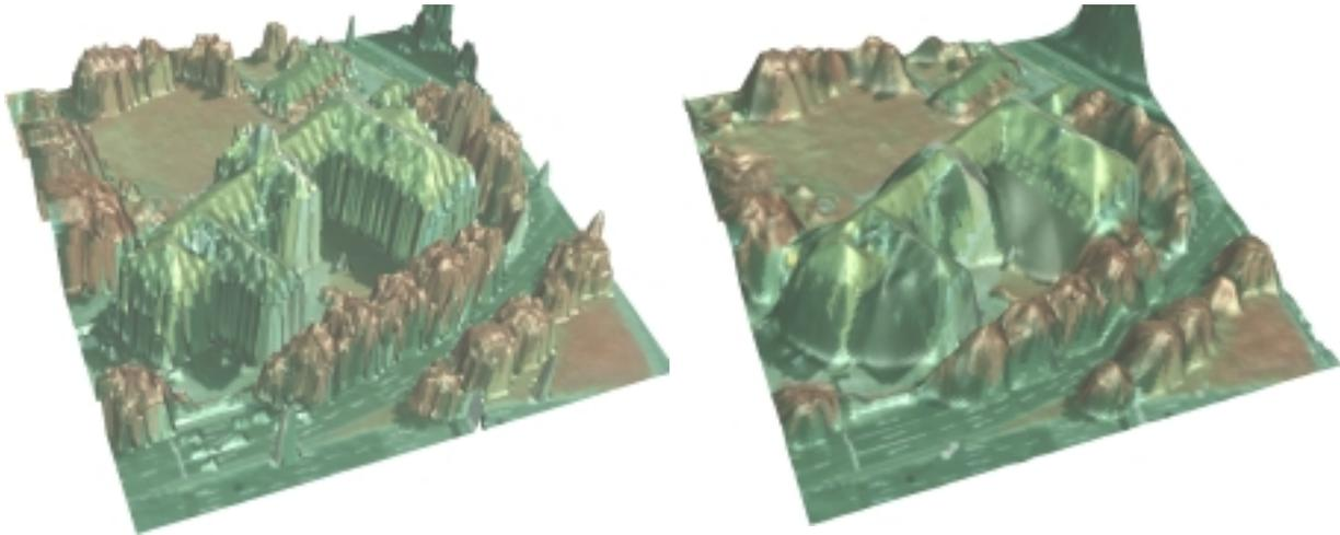
Figure 2: Comparison between a DSM from laser scanning (TopoSys scanner, left) and image matching (Match-T, right), shown as 3D visualization. Note that the laser scanner DSM appears to be much sharper.
