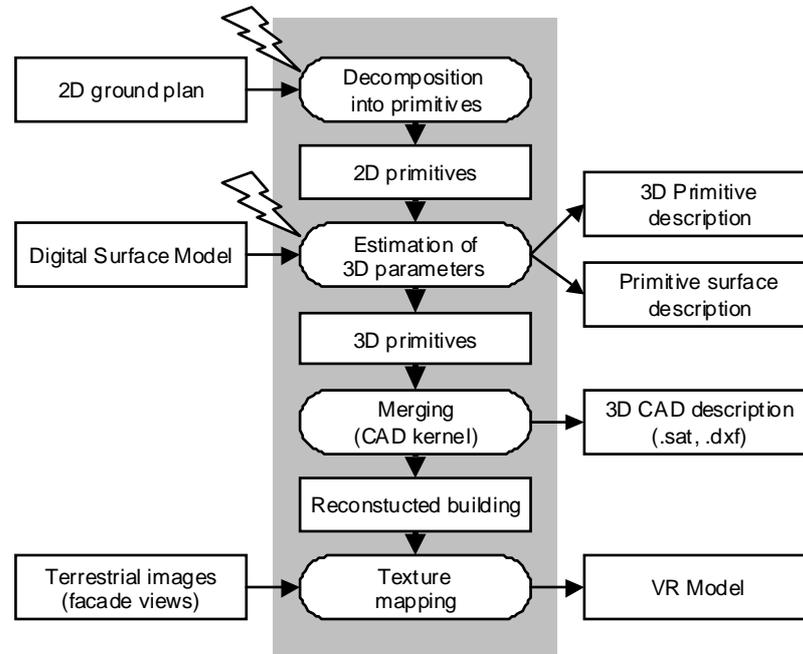
Figure 4: Workflow for the automatic and semi-automatic reconstruction algorithm.
