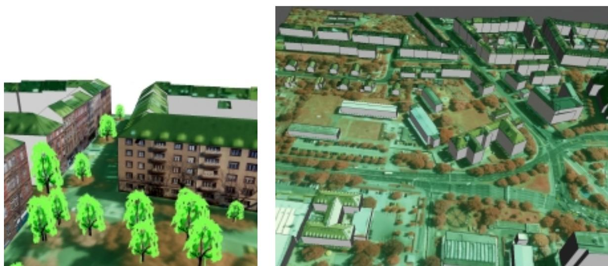
Figure 7: Texture mapped scenes (Karlsruhe dataset, 200 buildings). Left: Scene with facade texture taken from terrestrial images, roof texture taken from aerial image. Right: Larger scene with roof texture only.
