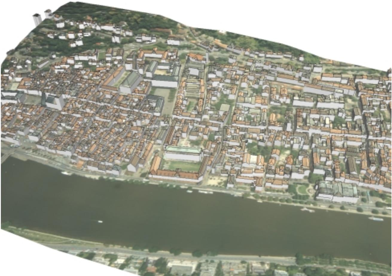
Figure 8: Automatically reconstructed buildings for the Heidelberg dataset (1400 buildings), with ortho image and roof texture from aerial image.
