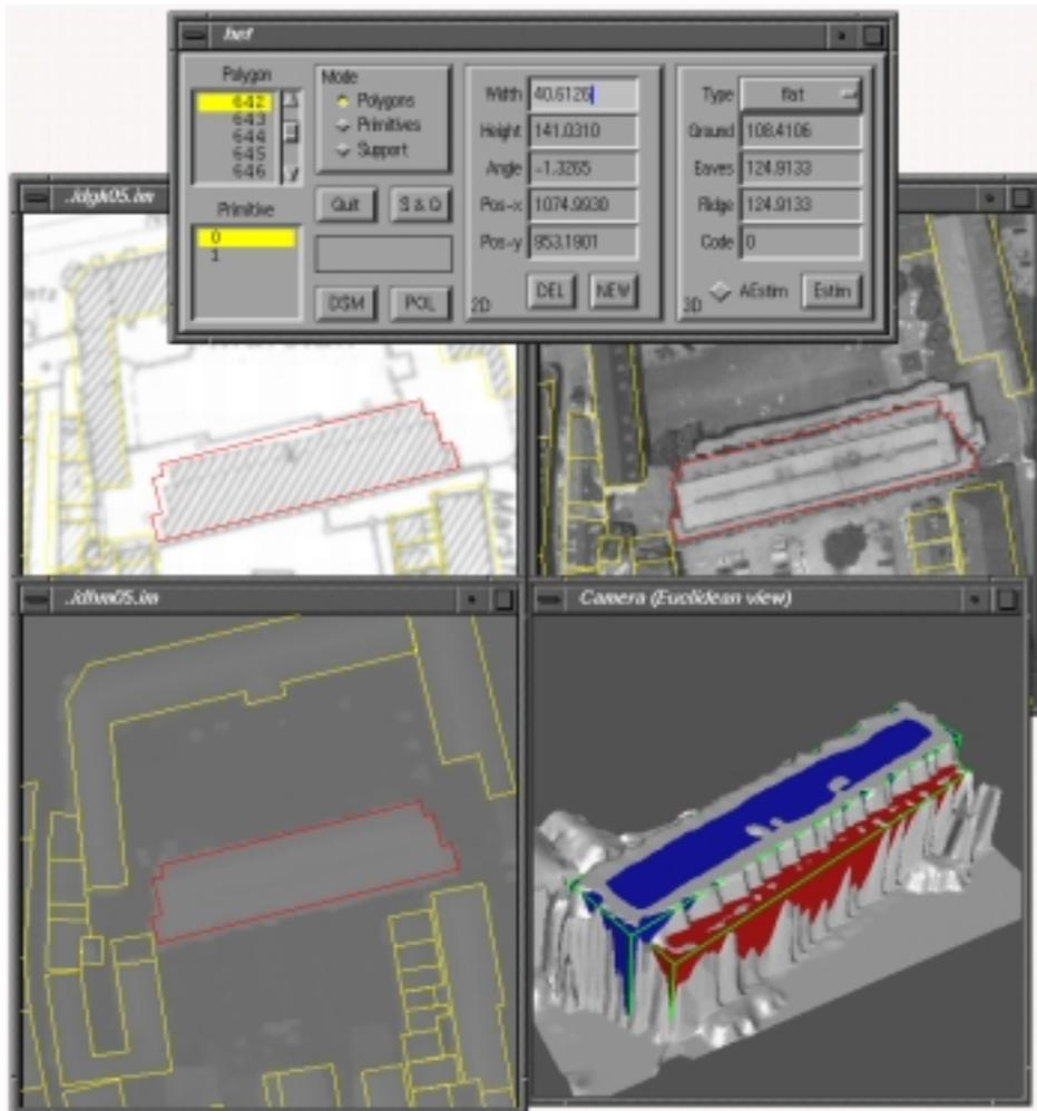
Figure 5: Interactive editing tool with map, ortho image, graycoded DSM and 3D view of DSM and reconstructed building.
