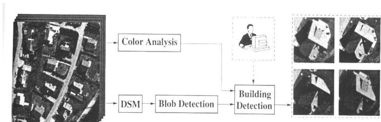
Figure 5: Our approach to automatic building detection. The method effectively combines color analysis with information extracted from elevation blobs in the DSM.
