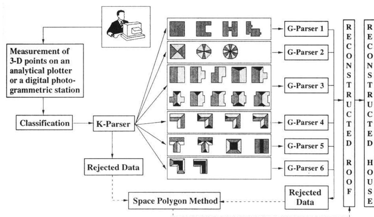
Figure 4: Structuring process of a point cloud into CAD-compatible 3-D roof models and complete buildings.
