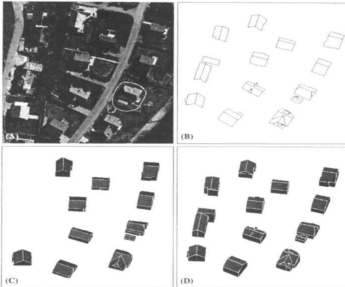
Figure 7: The results of 3-D reconstruction. (A) an original color image, (B) ground truth data, (C) fully automatic 3-D reconstruction using the ARUBA system, and (D) semi-automatic 3-D reconstruction using the TOBAGO software. The ground points (building heights) were manually set for the results in (D), whereas in (C) the DTM was used.
