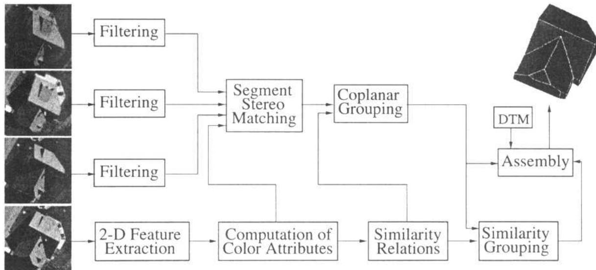
Figure 6: The ARUBA system for fully automatic 3-D reconstruction of buildings.
