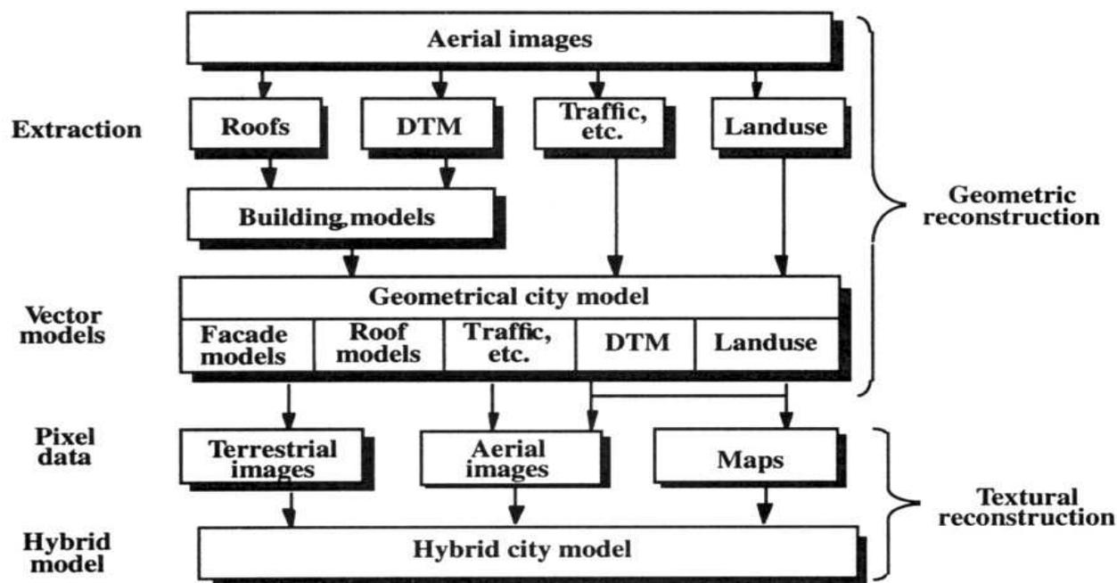
Figure 1: Generation and components of the geometric and radiometric parts of a hybrid city model.
