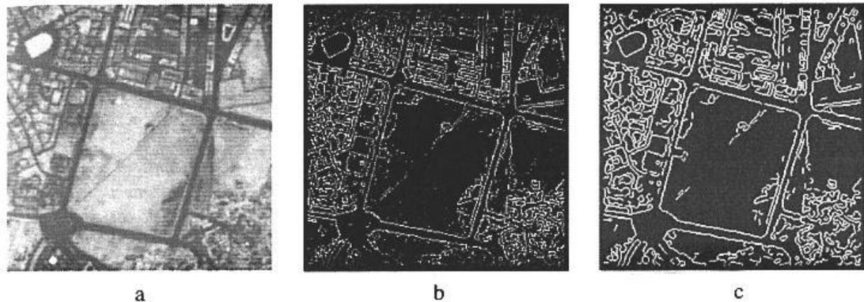
Figure 5: (a) MOMS-02 image of Dubai-City, (b) extracted edges, (c) derived lines.
