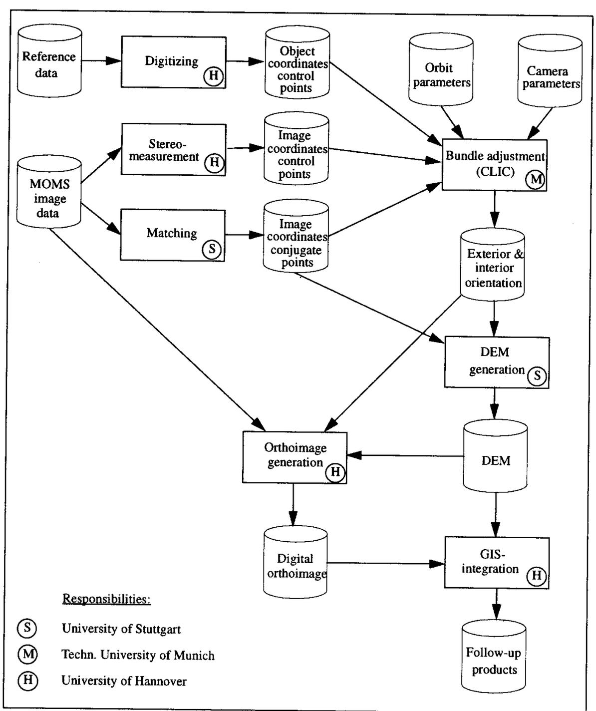
Figure 3: Digital photogrammetric data processing of MOMS-02/D2 data.
