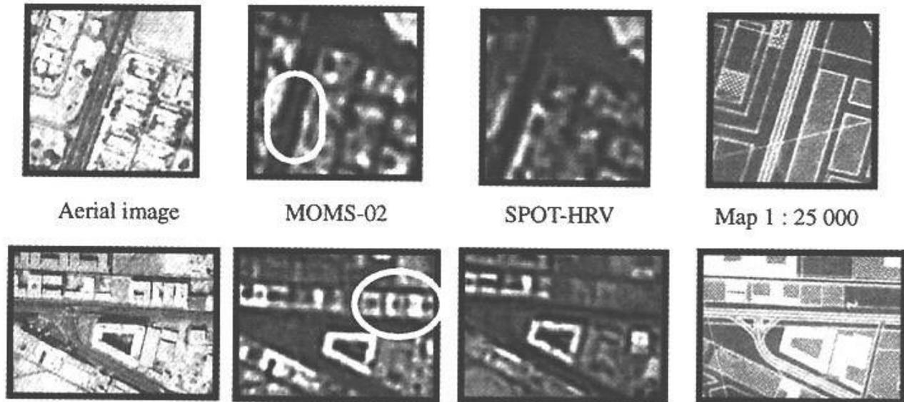
Figure 2: Comparison of the information content (brought to an unique scale).
