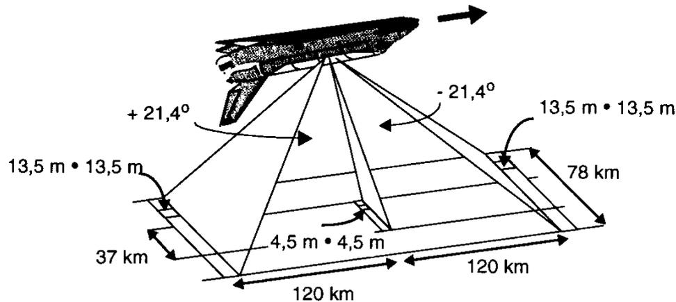
Figure 1: MOMS-02/D2 stereo imaging mode.
