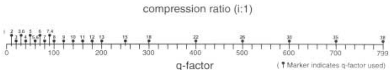
Figure 2: Approximate values of compression ratios for different q-factors.
