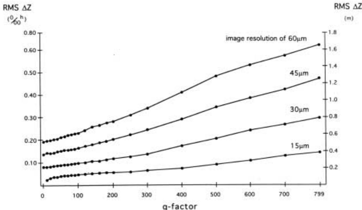
Figure 4: RMS heighting errors relative to the 15  $\mu\text{m}$  benchmark DTM for JPEG compressed images at four resolutions.
