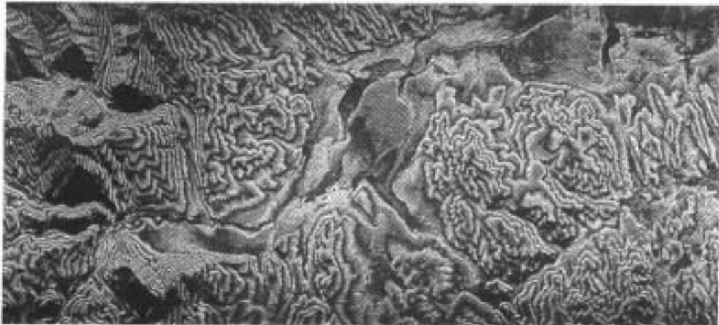
Figure 6: Interferometric SAR gray scale contours (3-levels) from INSAR interferogram. Bow Valley, Alberta, just west of Calgary. Courtesy of Canada Centre for Remote Sensing.
