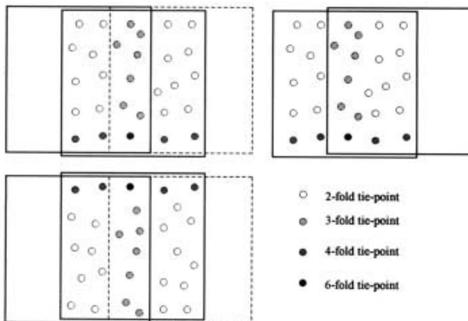
Figure 2: Tie-point locations in multiple overlapping images.
