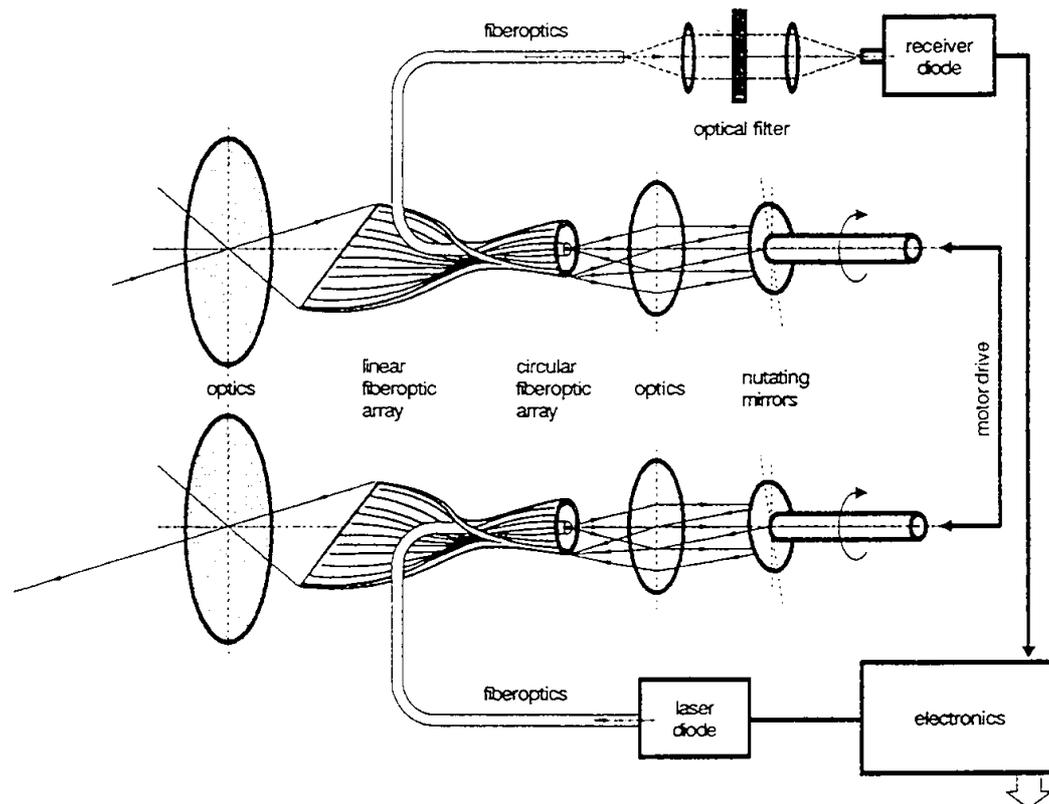
Figure 2: Architecture of the Laser Scanner.
