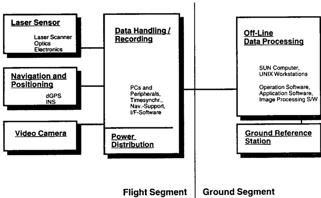
Figure 1: TopoSys System Components.
