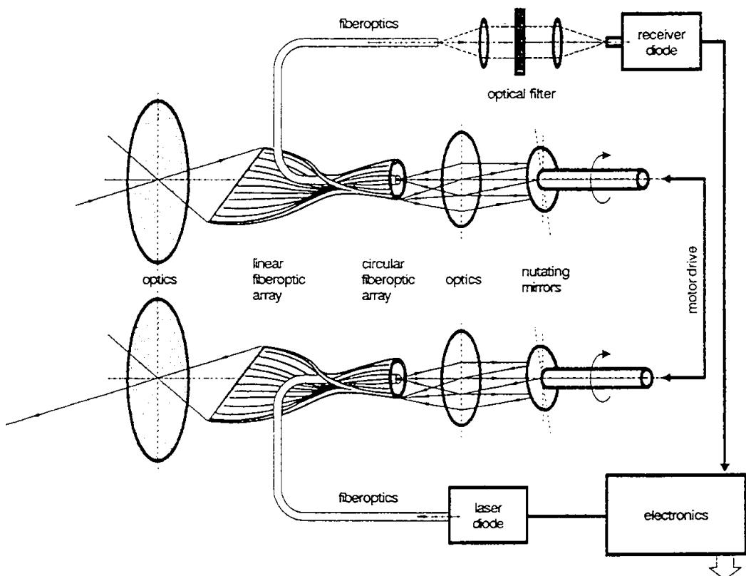
Figure 2: Architecture of the Laser Scanner.
