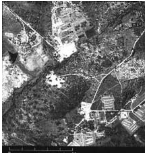
Figure 3b: MOMS-02 panchromatic band. GIFOV: 4.5m x 4.5m. Range: 512nm-765nm. Linear stretch, histogram cut-off at \pm 2.5\sigma . Note the increasing apparent albedo and transparency of vegetated areas.
