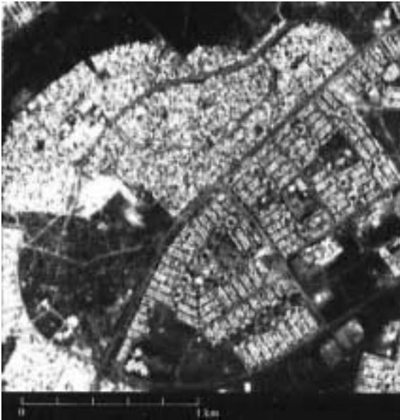
Figure 2a: HRV panchromatic band of high density suburb south of Harare. GIFOV:10m x 10m. Range: 510nm-730nm. Linear stretch, histogram cut-off at \pm 2.5\sigma .
