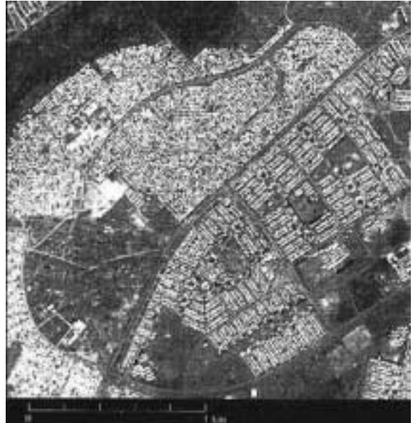
Figure 2b: MOMS-02 panchromatic band. GIFOV: 4.5m x 4.5m. Range: 512nm-765nm. Linear stretch, histogram cut-off at \pm 2.5\sigma . Note the increasing apparent albedo and transparency of vegetated areas.
