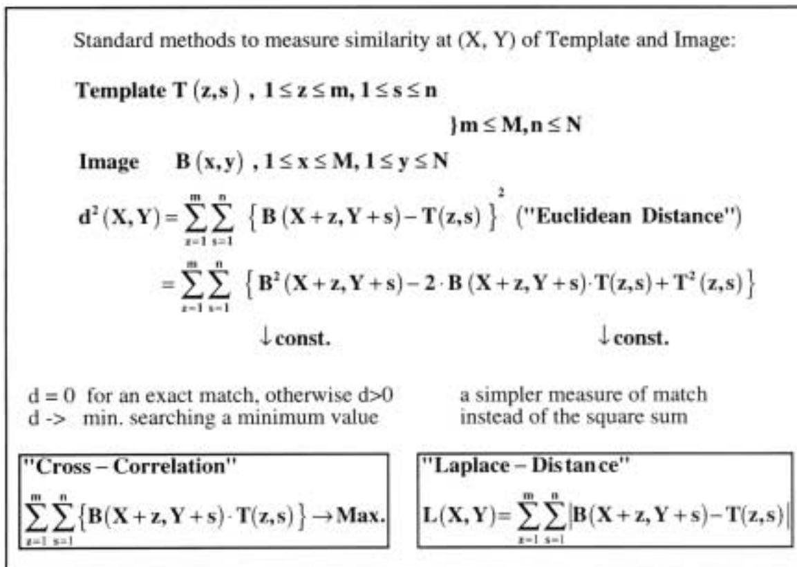
Figure 4: Similarity measure by "Cross-Correlation" or "Laplace-Distance".
