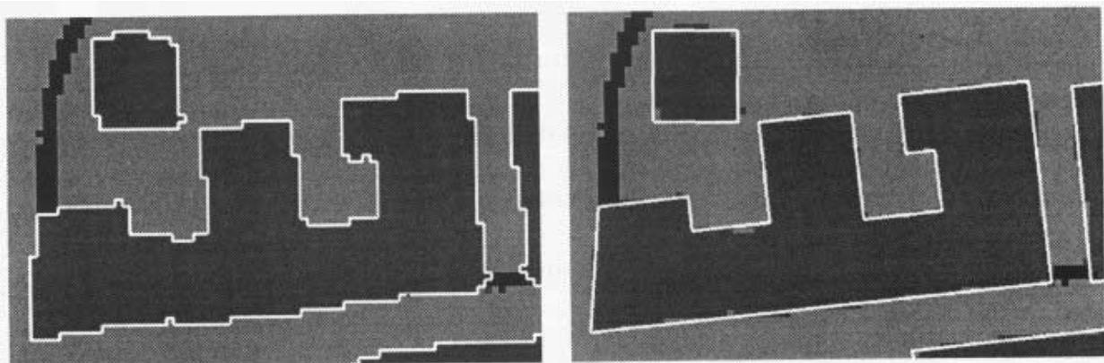
Figure 6: Raw contour polygons and automatically adjusted object contour segments (using geometric constraints and robust estimators).
