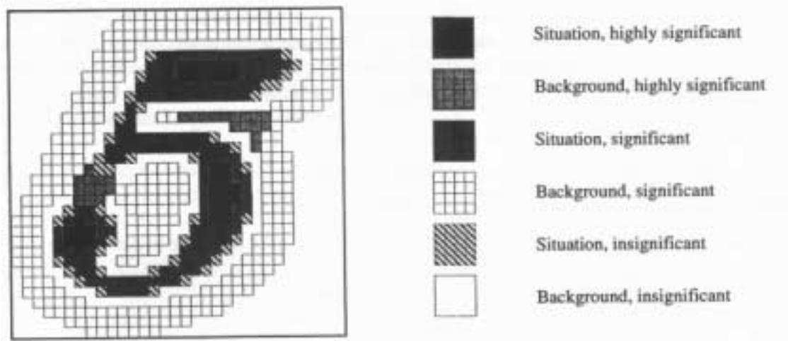
Figure 5: Template definition with significance levels.
