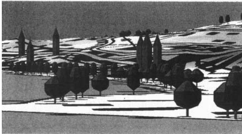
Figure 7: 3D-Visualisation of the map 1:25 000 with automatically recognized trees and towers.
