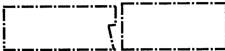
Figure 7: Unfavorable distribution of the pattern elements to the left; clear angles to the right.
