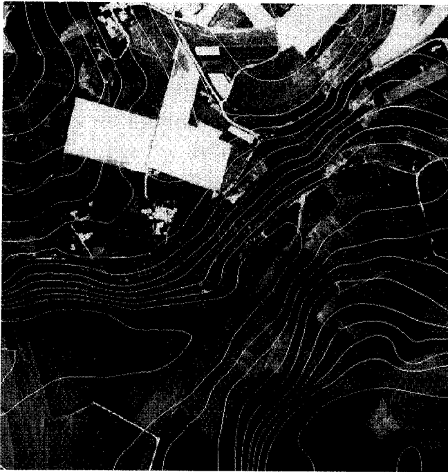
Figure 8: Orthophoto with contour line overlay
