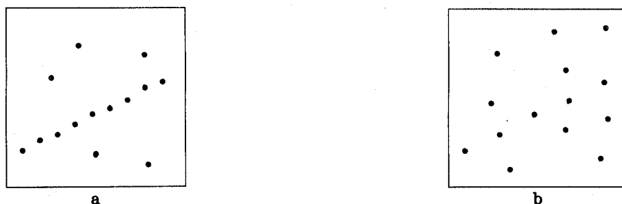
Fig. 2.1 14 points within a square, most likely interpretations: a) 9 points on a straight line and 5 outliers b) random set or 5 points on a straight line and 9 outliers?
