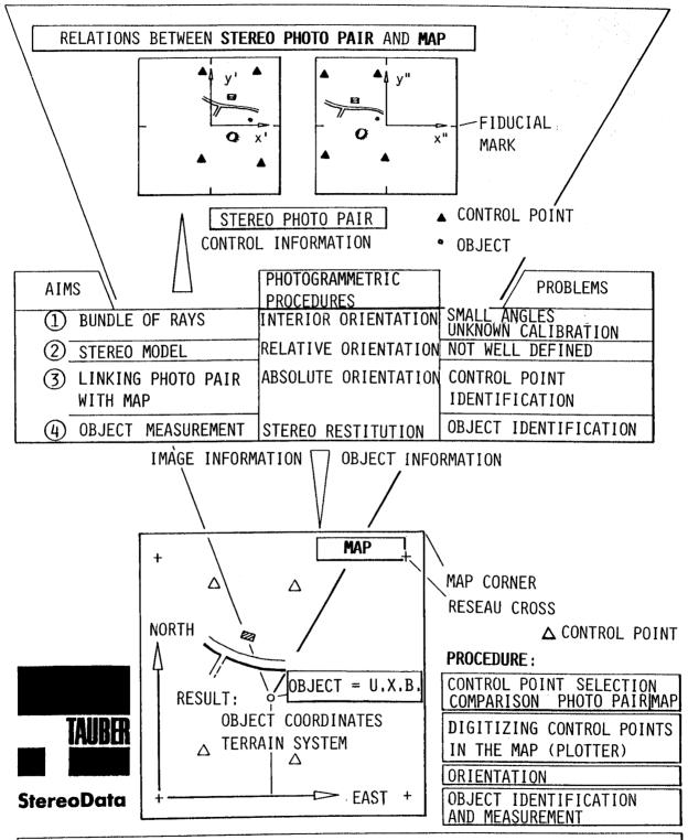
INTERCONNECTION OF STEREO PHOTO PAIR AND MAP BY AFFINE TRANSFORMATION USING UP TO 9 MAP CROSSES OR MAP CORNERS AND UP TO 25 CONTROL POINTS
