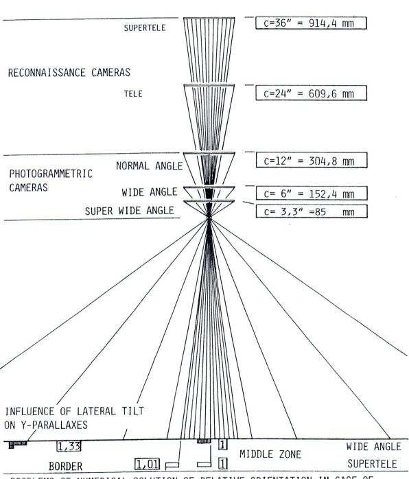
PROBLEMS OF NUMERICAL SOLUTION OF RELATIVE ORIENTATION IN CASE OF SUPERTELE STEREOMODELS — SMALL BUNDLE OF RAYS —
