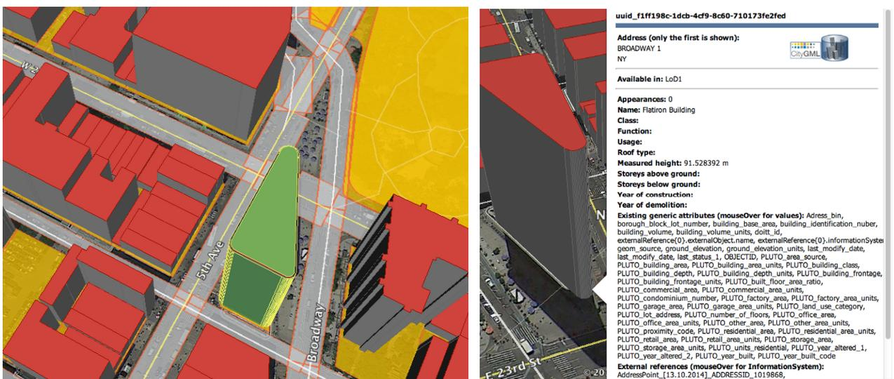
Figure 9: Screenshot showing the 3D city model of Manhattan where 5<sup>th</sup> Avenue meets Broadway. Left image: LOD1 buildings, LOD1 street surfaces (light grey), land parcels (yellow). Right image: list of attributes attached to the CityGML building model of the famous ‘Flatiron Building’. These can be queried and used for further analyses.
