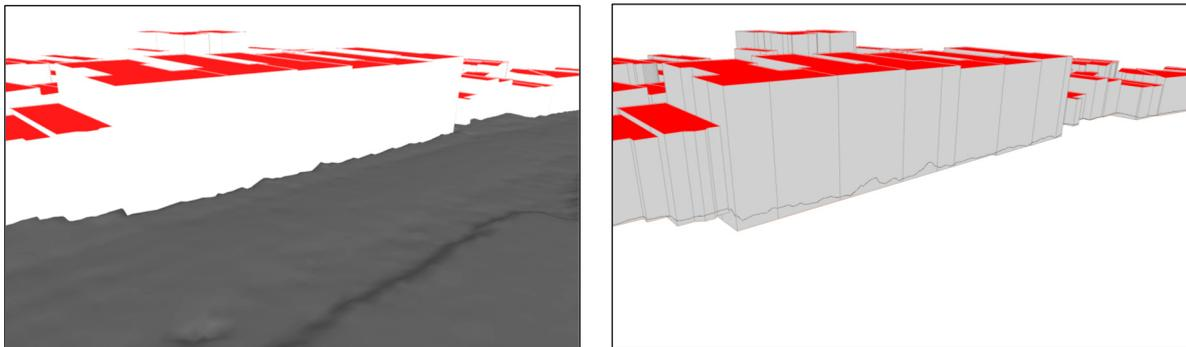
Figure 3: Left: generated 3D building objects shown together with the DTM. Right: terrain intersection curves (TIC) are 3D rings around the building solids denoting the intersection line with the terrain.
