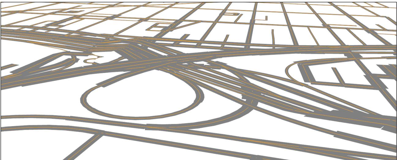
Figure 7: Road network and road surfaces of a complex motorway junction mapped to the DTM. Local heights are varied for bridges and elevated roads according to their different height levels. For road sections linking different height levels the height values are linearly interpolated along the centerline.
