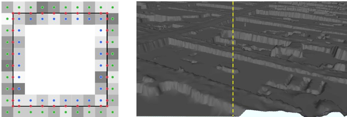
Figure 2: Left: DTM height points considered in computing the boundary height profile for each TIN tile. Blue points belong to height values from cells within the tile and green points lie outside. From the blue and green points the heights of the red points are interpolated. The tile boundaries (black lines) are used as break lines in the triangulation. Right: visualization of two adjacent TIN tiles (the boundary is indicated by the yellow dashed line).
