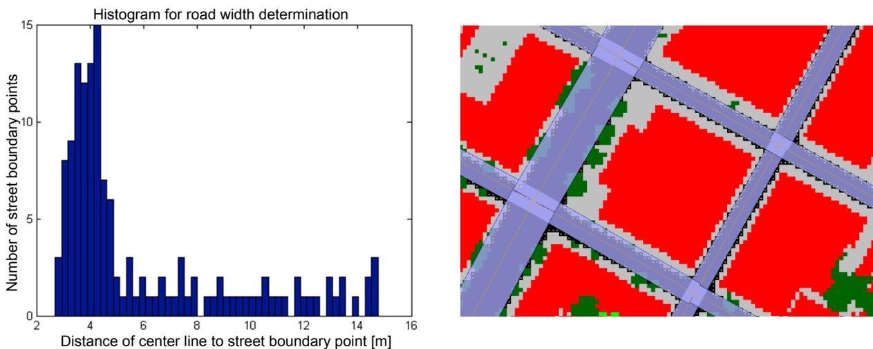
Figure 5: Left: Histogram of computed distances from sample points along a street center line to the last land cover cell classified as 'street' in transversal direction. Right: 2D street surface polygons (in blue) created from buffering the center lines with the estimated street width.
