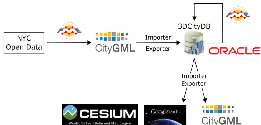
Figure 8: Workflow and employed tools. The source data from the NYC Open Data Portal is integrated and transformed to CityGML files using FME and imported into the 3DCityDB. Then the 2D-3D transformations are carried out in the geodatabase. The final results are exported to CityGML files for further applications and to KML files for visualization.
