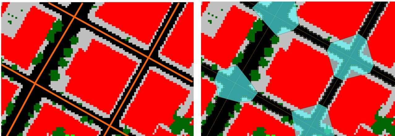
Figure 4: Road network (in orange colour) overlaid onto the land cover classification raster dataset. Red areas denote buildings, black areas streets, green areas vegetation, and grey areas pedwalks or other paved areas. The right image shows the automatically determined street intersection areas (light blue) and street boundary points (yellow dots).
