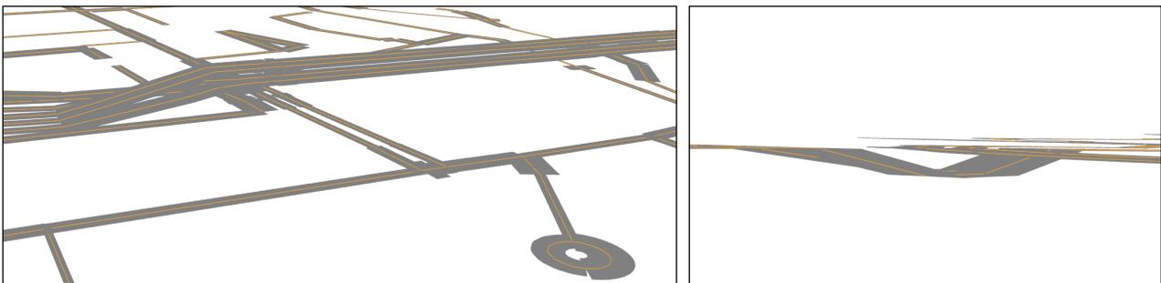
Figure 6: Road network and road surfaces mapped to the DTM. Local heights are varied for bridges and elevated roads (left) and tunnels or underpasses (right). Due to the lifting or lowering of road heights, road center lines or road surfaces that do not intersect in reality do not intersect spatially in the resulting CityGML 3D dataset either.
