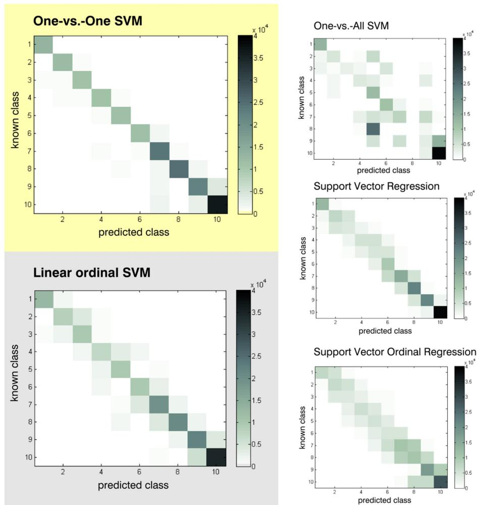
Figure 3: Confusion matrices of the investigated prediction algorithms. The one-vs.-one SVM is used as the golden standard because it represents the capable and flexible model. The Linear Ordinal SVM achieves comparable results with much lower model complexity and out-performs the three other models.
