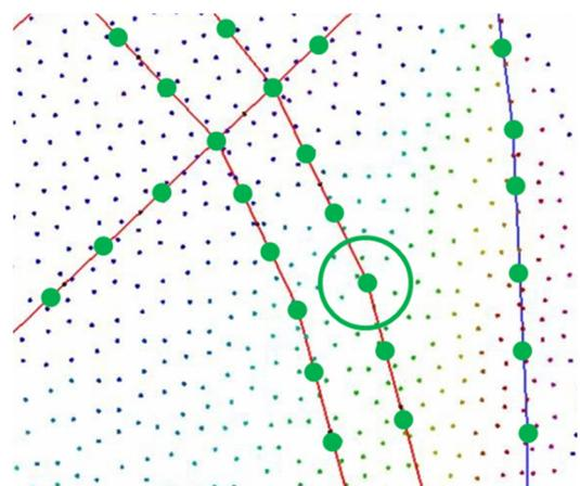
Figure 2: Local object heights are determined at locations of the 2D polygon nodes as well as many nodes inserted in between.
