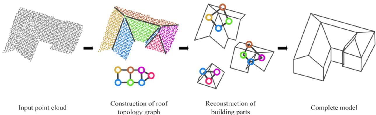
Figure 5: The topology of segmented roof point clouds serves to recognise shapes of roof parts.
