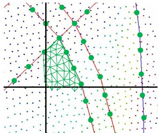
Figure 3: In each tile object surfaces are modelled by triangles up until the tile boundary.
