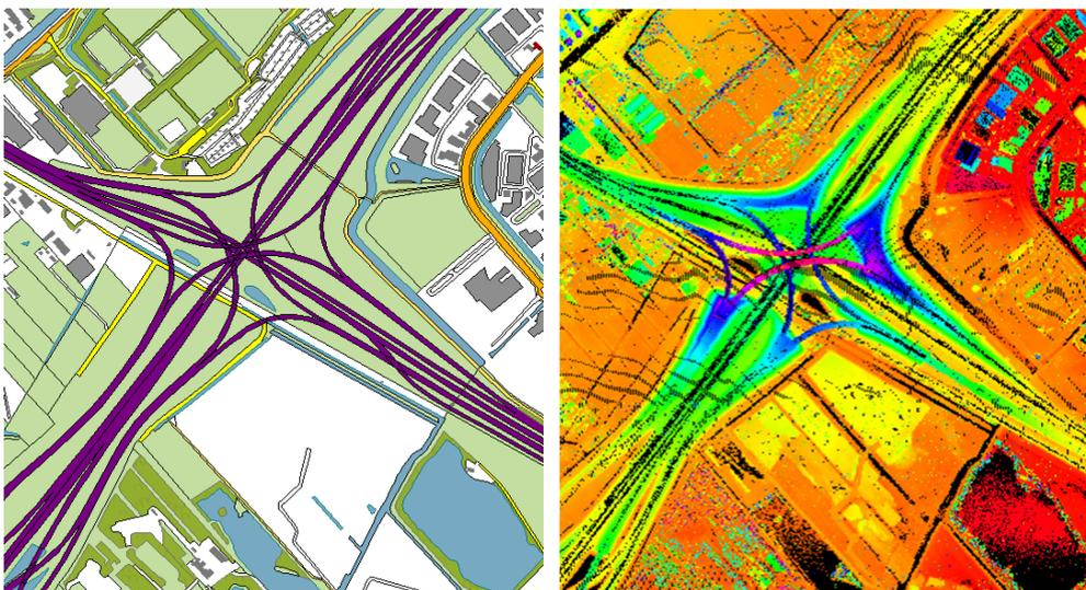
Figure 1: Example of the TOP10NL and (height coloured) AHN data.
