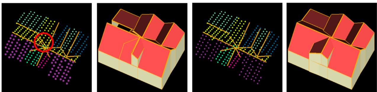
Figure 6: Correction of detected roof topology. Left: incorrect detected intersections of roof faces and the corresponding wrong model. Right: corrected intersections and model.
