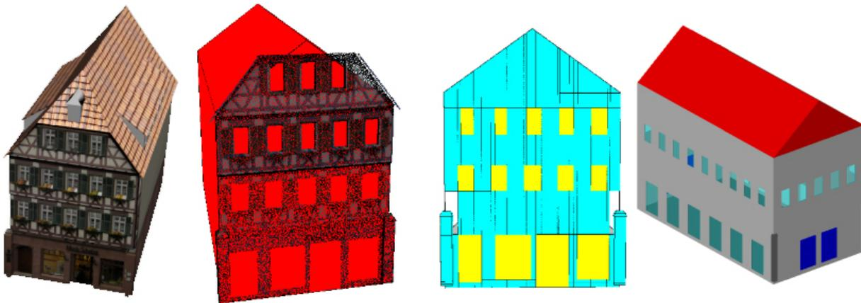
Figure 4: From Left to Right: Textured model of the Hermann Hesse birthplace, simplified CityGML model with an overlying point cloud, reconstructed primitives, bottom right: grammar based completion.
