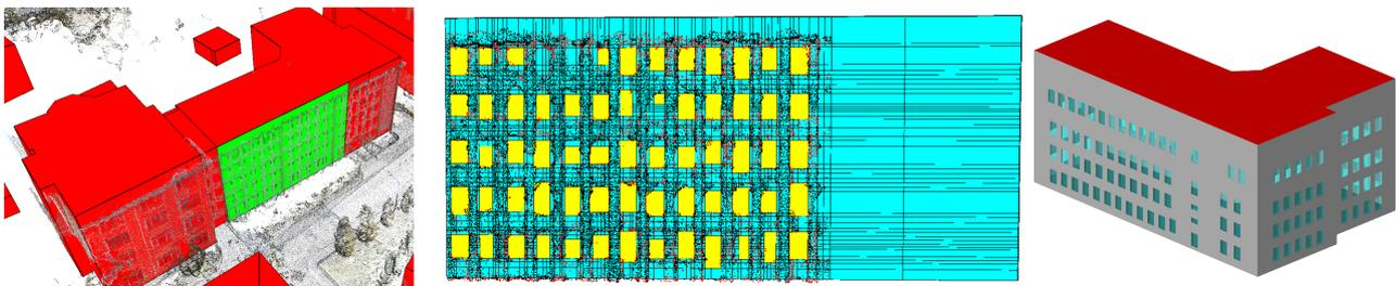
Figure 3: From Left to Right: Coarse building model with selected façade of interest, 3D cell decomposition with reconstructed primitives, enriched CityGML LoD3 model.
