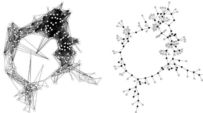
Figure 2: Reducing the full match graph (left) to a skeletal set (right) greatly reduces the number of image pairs that need to be matched, while nevertheless preserving an acceptable camera network for reconstruction.
