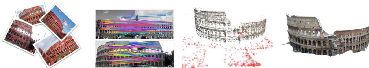
Figure 1: The 3D modeling pipeline. Interest points are extracted and matched to obtain tie-points. The tie-points enable (relative) image orientation. Finally a (optional) dense reconstruction recovers a point cloud or surface model.
