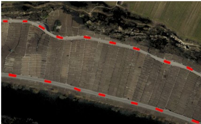
Figure 7: Planar test areas to determine the relative accuracy (std.dev., noise) of DSM (vertical component). Not all the defined polygons, only those in centre part of the test areas are shown.
