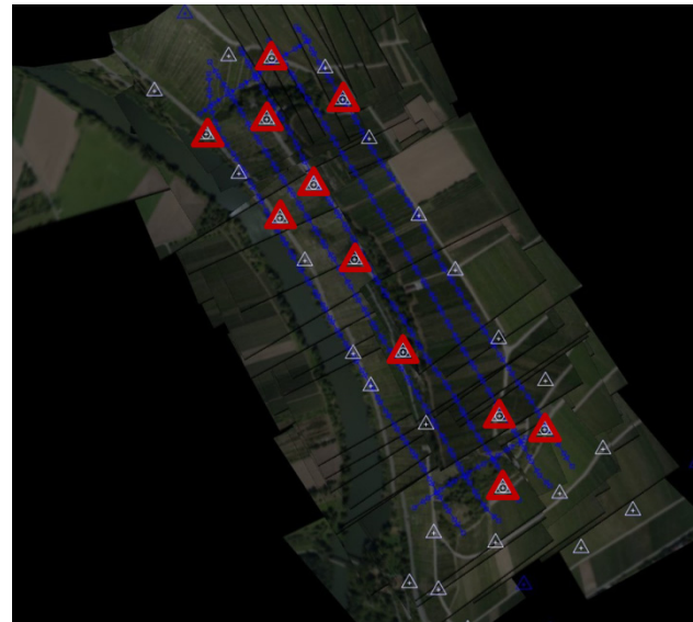
Figure 2: Hessigheim ground control and check point configuration (as used in later processing). Check points are highlighted in red.
