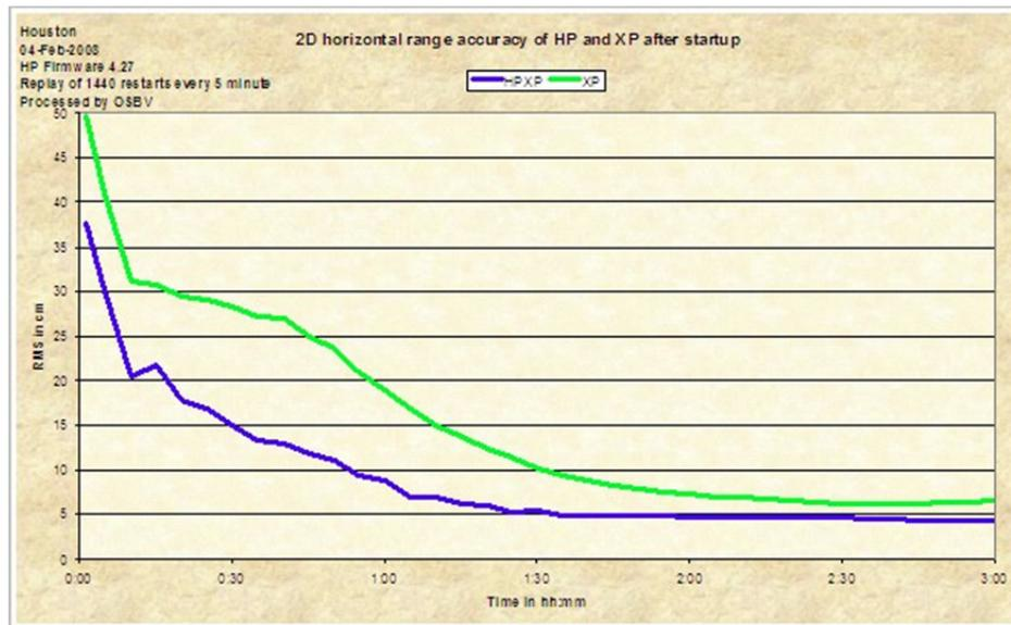
Figure 6: Standard deviation of horizontal accuracy after start-up for HP<sup>+</sup> (HPXP) and XP only [13]
