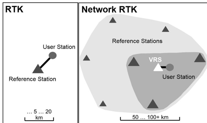
Figure 2: Principles of RTK and Network RTK from [16]
