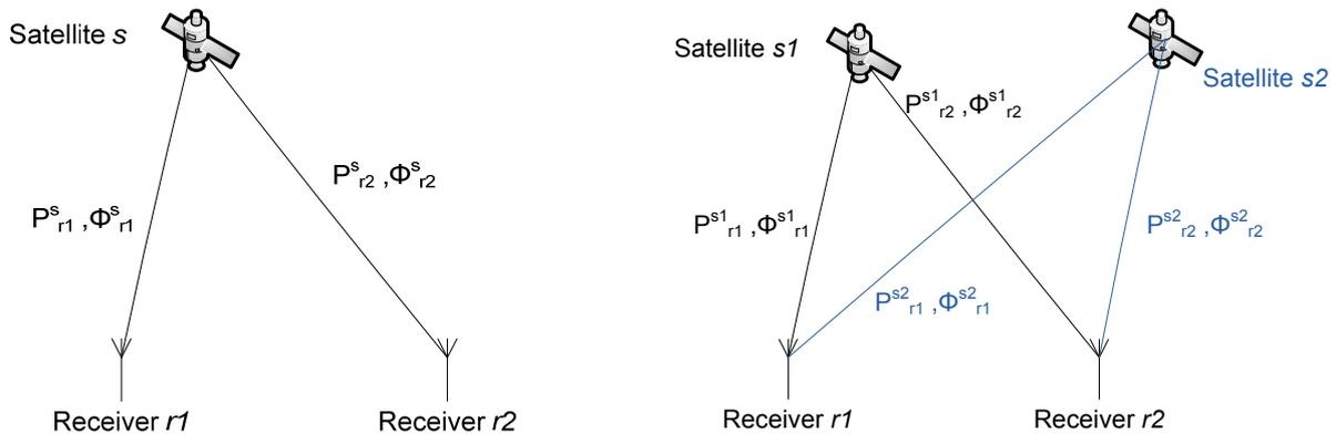
Figure 1: Visualization of single- (left) and double-differences
