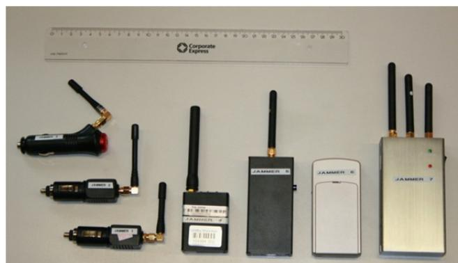
Figure 8: Examples for commercial InCar Jammers [1]
