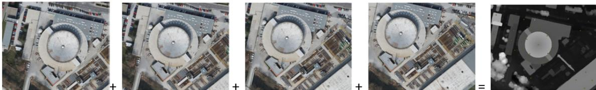
Figure 5: A series of high-overlapping 10cm GSD images resulting in a dense surface model (>50 points per square meter) through automated dense matching
