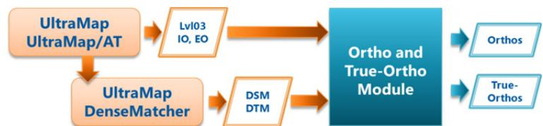
Figure 7: UltraMap Ortho/True-Ortho module.
