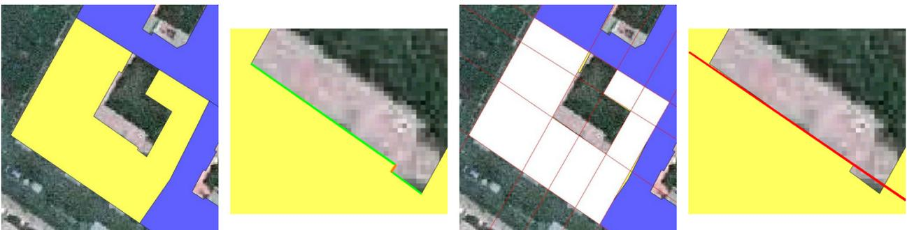
Fig. 3: Overview and close-up view of a building footprint (left) and its cell decomposition (right).
