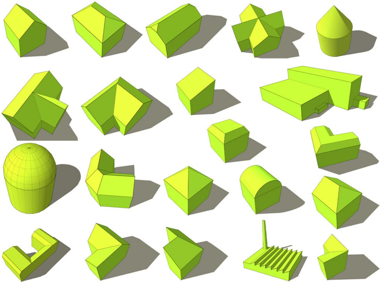
Fig. 4: A selection of elemental roof shapes and their combination to more complex building models.
