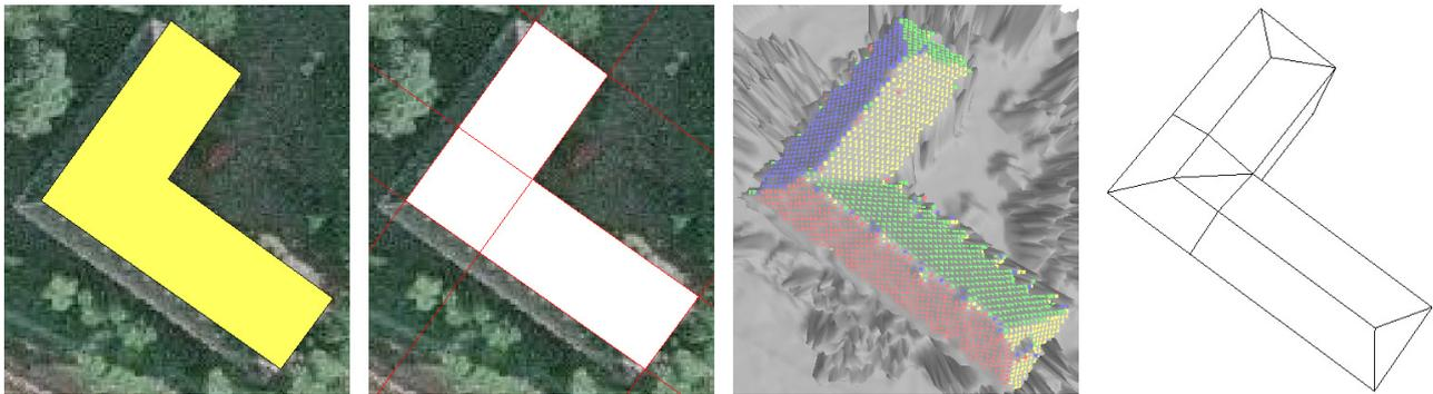
Fig. 2: The reconstruction algorithm decomposes a given building footprint (1) into mostly quadrilateral cells (2), classifies the LIDAR points according to their local regression planes (3) and gives the cells the best fitting roof shapes (4).
