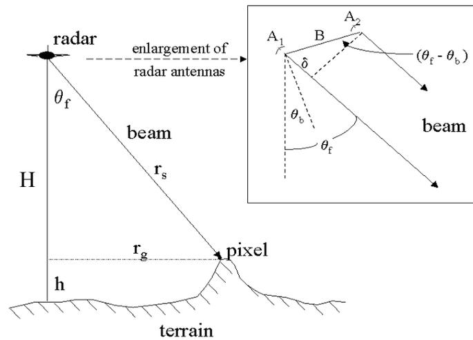
Fig. 1: Schematic of Airborne InSAR Geometry.
