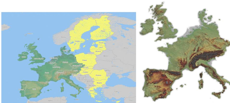
Fig. 3: Left: Outline of the current data-base coverage of NEXTMap Europe including the 15 countries listed in the text. Right: DSM of the area comprising approximately 2.2 million km<sup>2</sup>.
