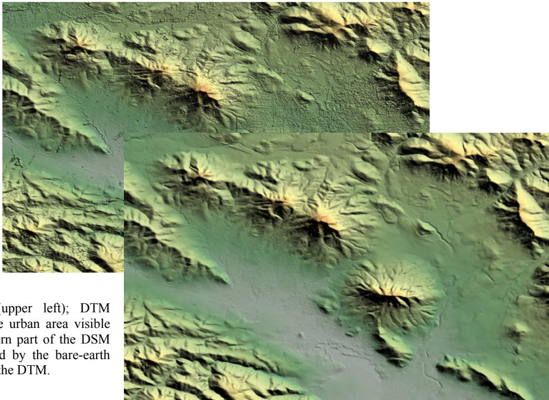
Fig. 4: DSM (upper left); DTM (lower-right). The urban area visible in the north-eastern part of the DSM has been replaced by the bare-earth representation in the DTM.
