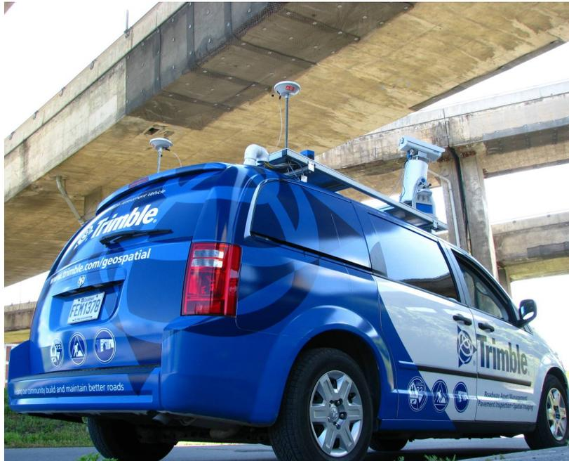
Fig. 3.2: Trimble Cougar Mobile Mapping System Image Courtesy of Trimble Navigation Ltd.
