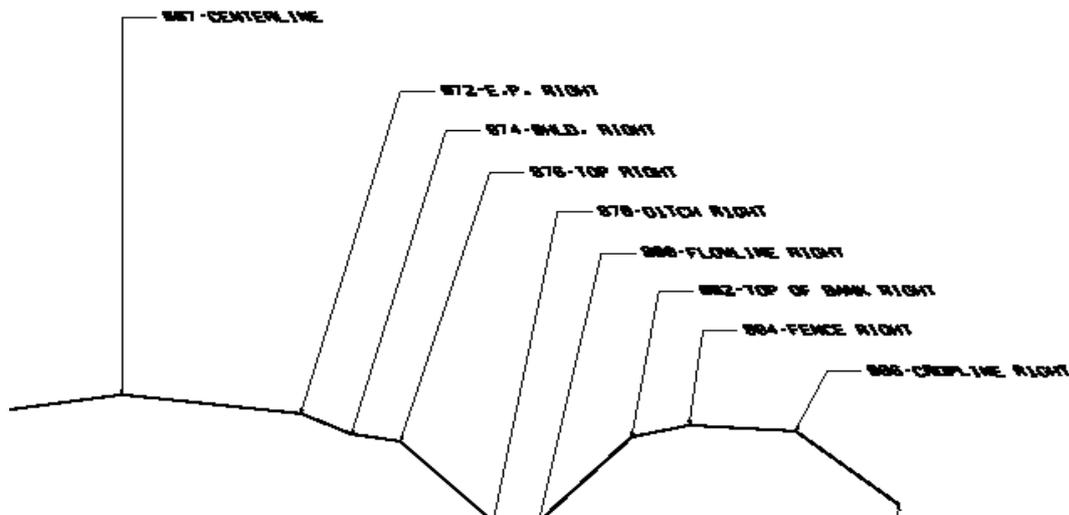
Fig. 3.1: Survey Field Coding Image Courtesy of Illinois Department of Transportation.
