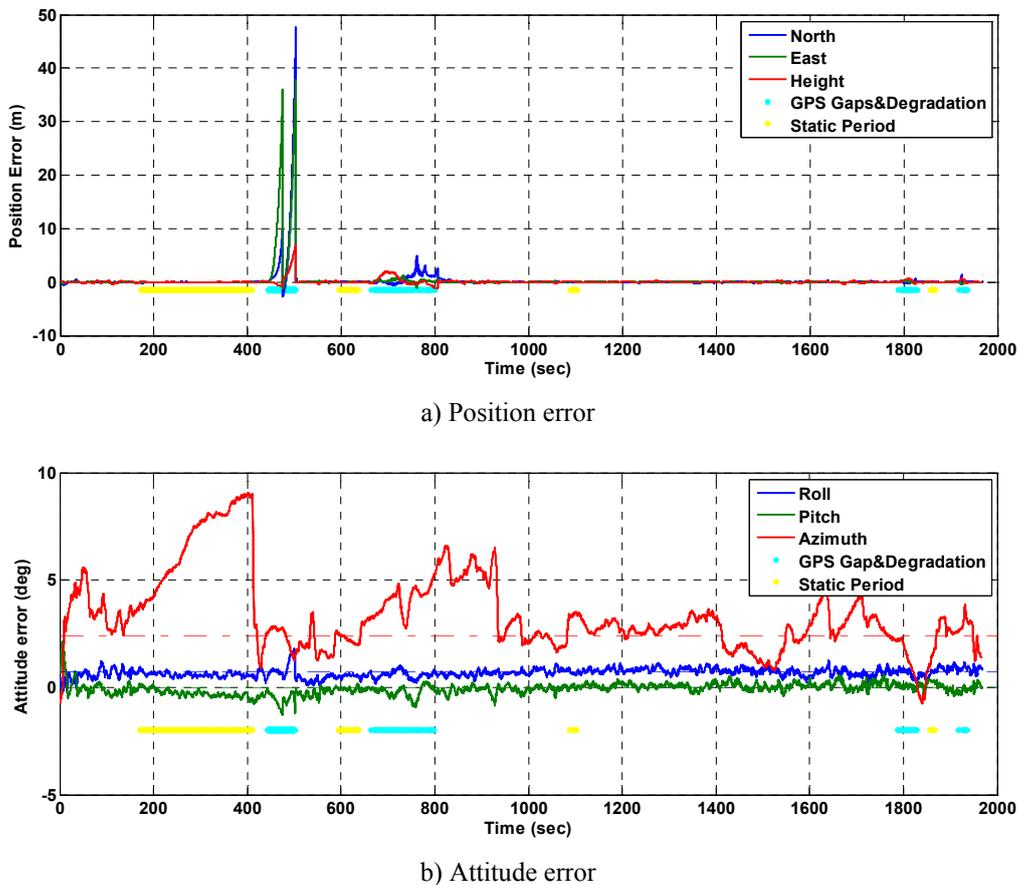
Fig. 4: Navigation error of the forward filtering.
