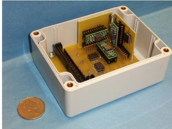
Fig. 1: MEMS IMU using sensors from ADI.
