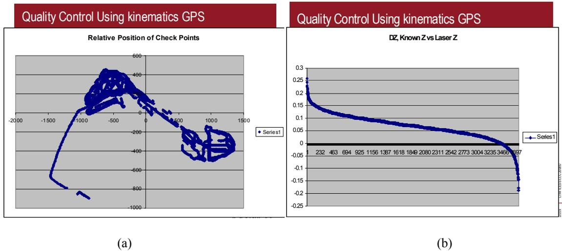
Fig. 8: (a) the navigation route of the car with GPS antenna (b) vertical error variances of the generated DTM compared to GPS points.
