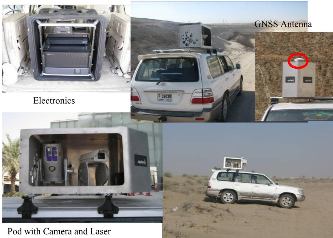
Fig. 5: The Land Mark System mounted on Land cruiser car.
