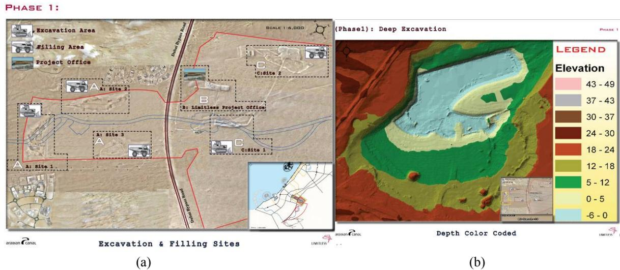
Fig. 7: (a) Details of the Excavation and filling sites along the canal route within Phase I of the development area. (b) 3D color coded image of the excavation site 1 shown in (a).
