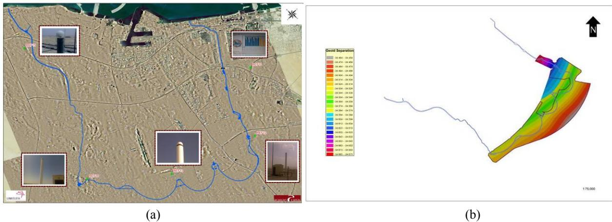
Fig. 3: Vertical Datum modeling and Distribution of five GPS/GNSS reference stations around the Canal and development area. (a) Location of the GPS/GNSS reference stations (b) Geoids' Model to model of the development area.
