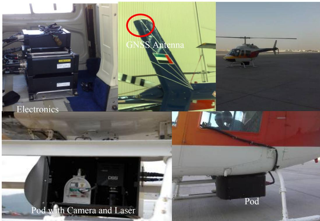
Fig. 4: The airborne System mounted in Bell 206.
