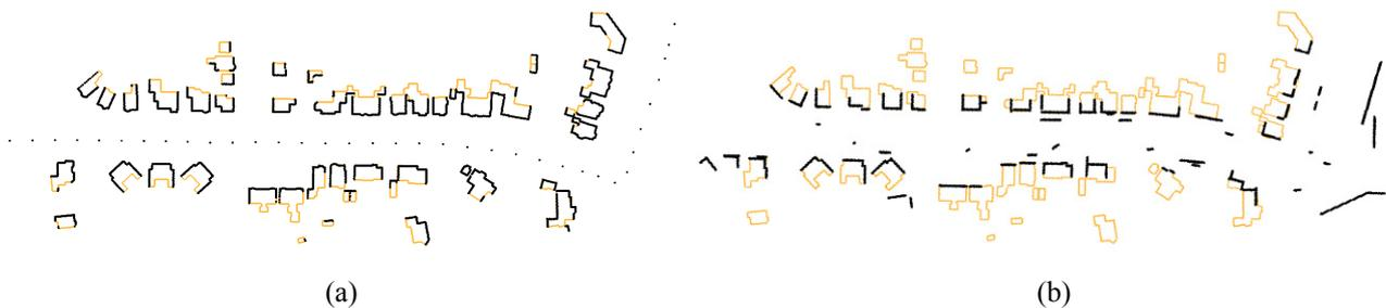
Fig. 5: (a) Theoretically visible walls and (b) automatically detected walls of a mobile laser scanning survey. The survey path is shown by dots. The yellow (light grey) lines are taken from the building layer of a large scale map.
