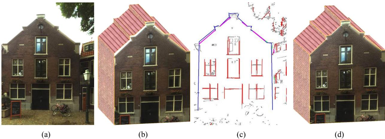
Fig. 7: (a) Image used for texturing, (b) Initial texture projection, (c) Extracted edges from model (blue) and image (red, pink), (d) Texture projection after adapting the model to the image edges.
