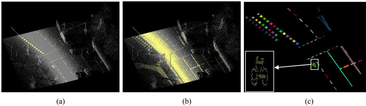
Fig. 4: (a) Point selected with high threshold on reflectance. (b) Points selected with low threshold on reflectance. (c) Detected road markings after distance dependent thresholding and connected component analysis.
