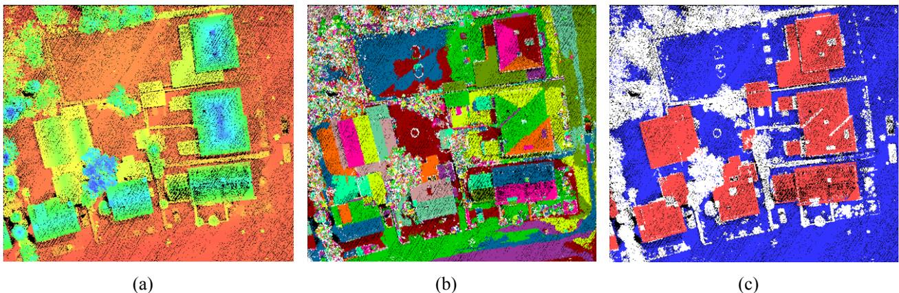
Fig. 1: (a) Point cloud with colour coded heights, (b) Point cloud segmented into planar surfaces, (c) Segments classified based on various segment properties (red (light grey): building, blue (dark grey): terrain: white: other classes).
