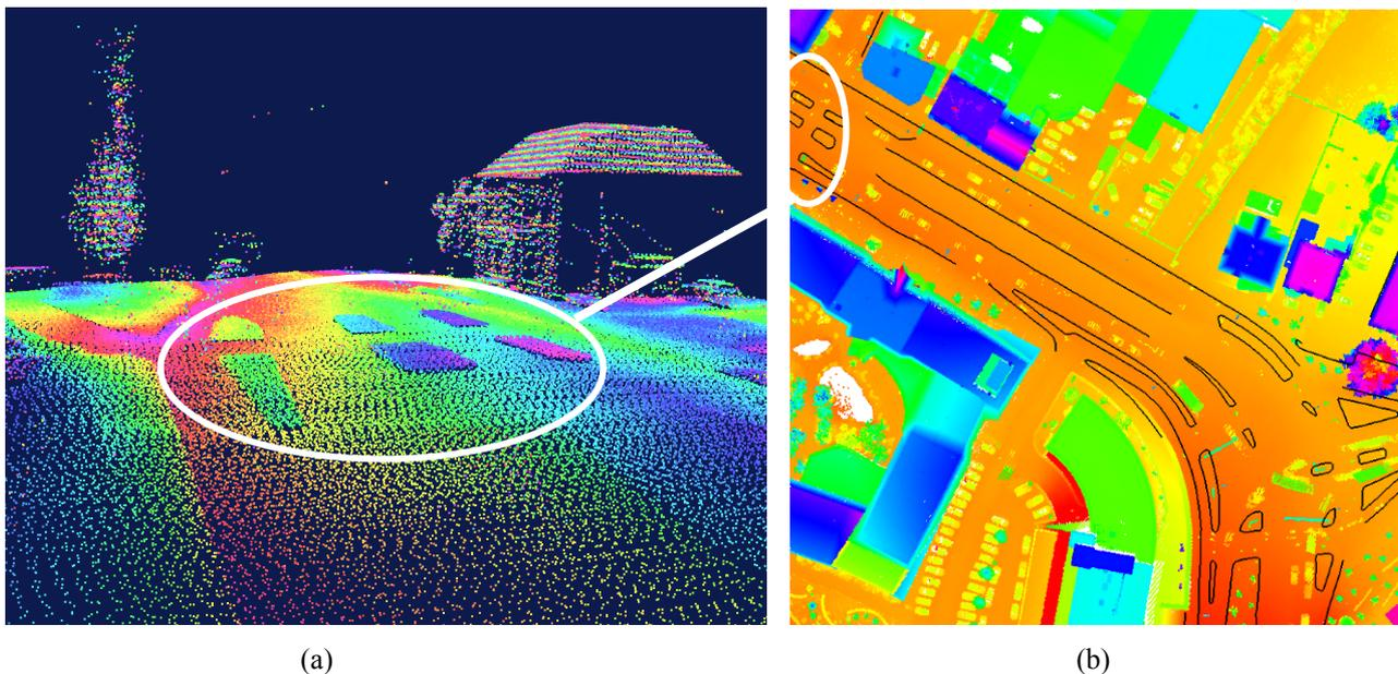
Fig. 3: (a) Perspective view of colour coded points showing small height differences of traffic islands.
