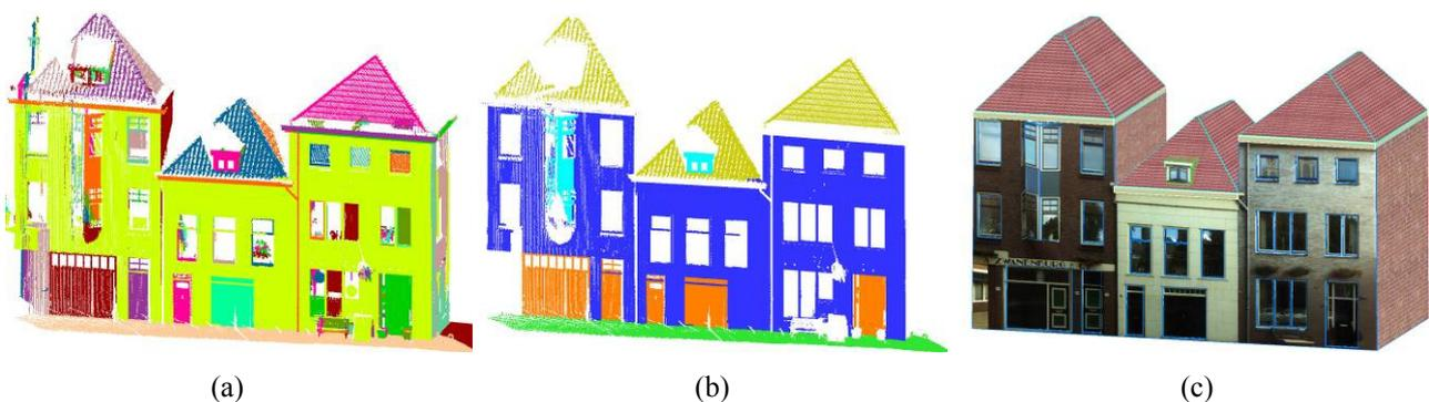
Fig. 6: (a) Segmented point cloud of a building façade. (b) Segments classified as wall (blue, dark grey), door (orange, grey), roof (yellow, light grey), protrusion (turquoise, light grey) or ground (green, grey). (c) Textured building model.
