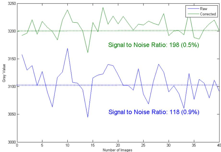
Fig. 6: SNR before and after aperture correction for 4.7 msec exposure time for a DMC image.
