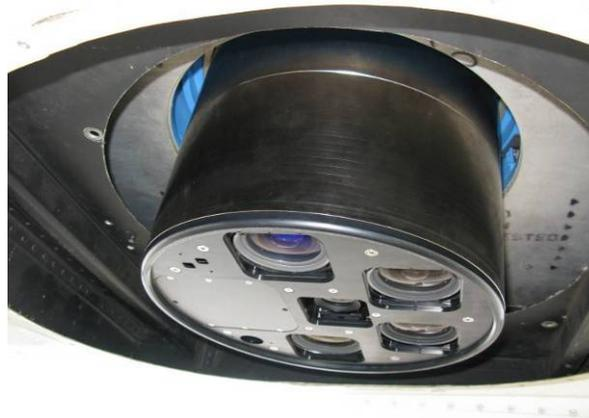
Fig. 1: RMK D front plate - view from bottom with 4 MS camera heads, video camera (center) and space for additional sensor (left).
