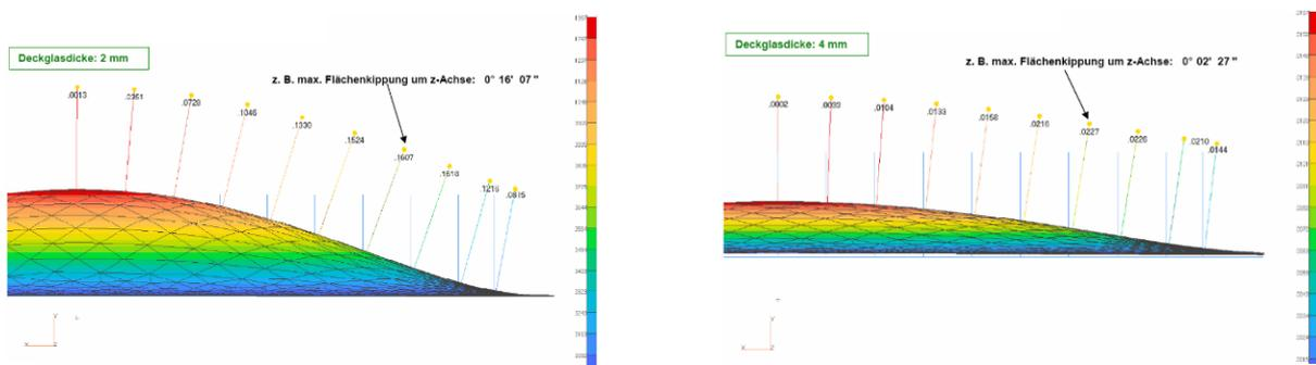
Fig. 3: (left) Deflection of a conventional 2 mm cover glass (max. tilt from z-axis 967) (right) RMK D – deflection of 4 mm cover glass resulting in max. tilt from z-axis of 147''.
