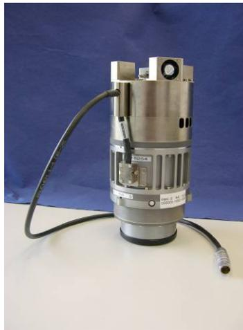
Fig. 2: RMK D – multi spectral camera head.
