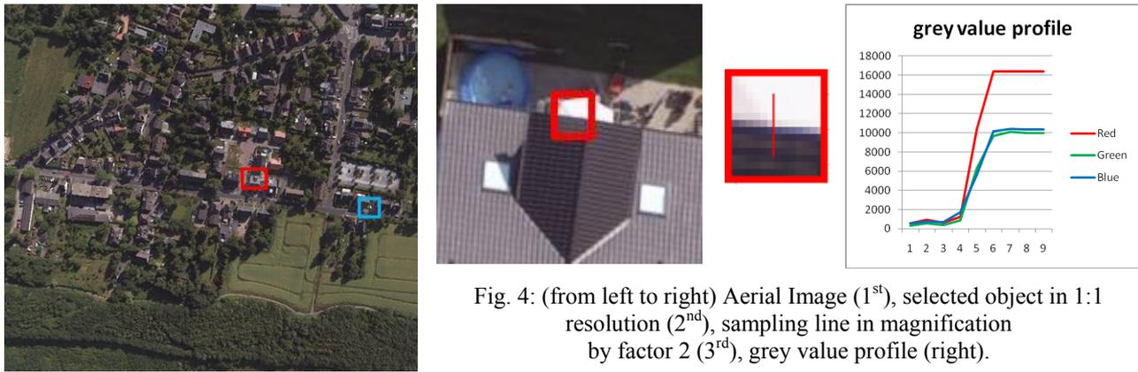
Fig. 4: (from left to right) Aerial Image (1<sup>st</sup>), selected object in 1:1 resolution (2<sup>nd</sup>), sampling line in magnification by factor 2 (3<sup>rd</sup>), grey value profile (right).
