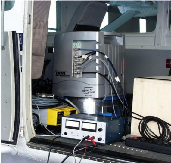
Fig. 5: DMC installed on an aircraft.
