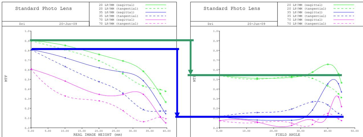
Fig. 14: MTF curves of a state-of-the-art photographic lens at different temperatures indicating 25% MTF decrease at half the Nyquist frequency of a 12um pixel sensor and 60% MTF decrease at half the Nyquist frequency of a 7.2um pixel sensor and 40K temperature change.
