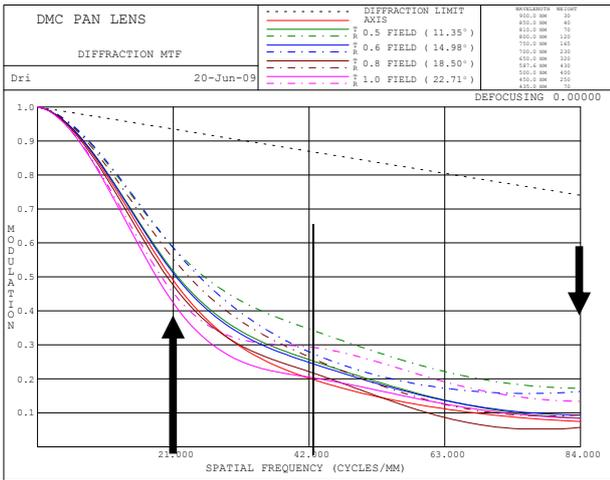
Fig. 6a: MTF as a function of  $\nu$  for 6 field points for DMC PAN Lens.
