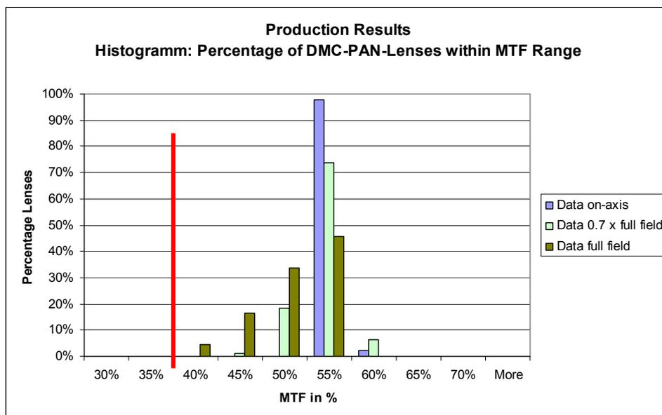
Fig. 16: Histogram of final measurement MTF performance for DMC – PAN lens.
