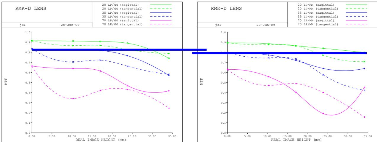
Fig. 13: MTF curves of the RMK-D Lens at different temperatures indicating 10% MTF change at half the Nyquist frequency (blue line) and 8000m height change.
