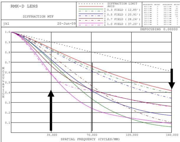
Fig. 7a: MTF as a function of  $\nu$  for 6 field points for RMK-D Lens.
