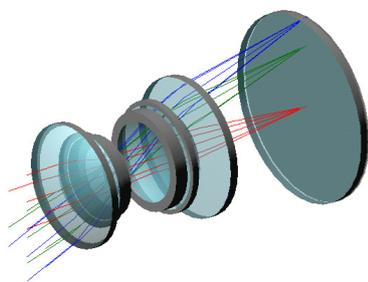
Fig. 5a: DMC PAN Lens.
