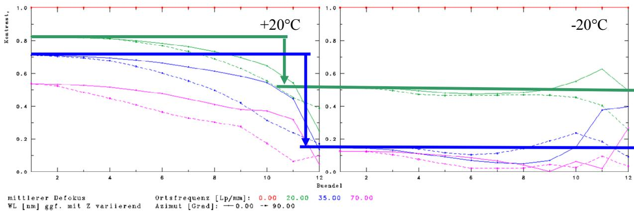
Fig. 11: MTF curves of a state-of-the-art photographic lens at different temperatures indicating 30% MTF decrease at half the Nyquist frequency of a 12um pixel sensor and 55% MTF decrease at half the Nyquist frequency of a 7.2um pixel sensor and 40K temperature change.
