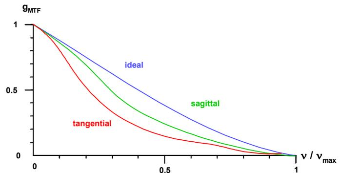
Fig. 4b: Modulation transfer for tangential and sagittal orientation of structures in the object and reference to the ideal transfer curve.
