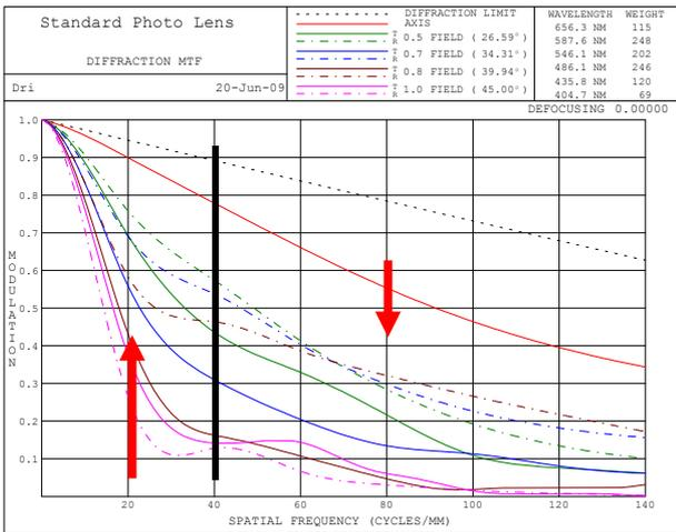
Fig. 8a: MTF as a function of  $\nu$  for 6 field points for state of the art photographic lens.
