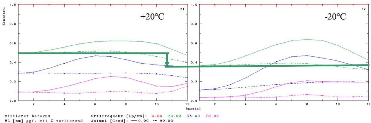
Fig. 9: MTF curves of the DMC Pan Lens at different temperatures indicating 15% MTF decrease at half the Nyquist frequency and 40K temperature change.
