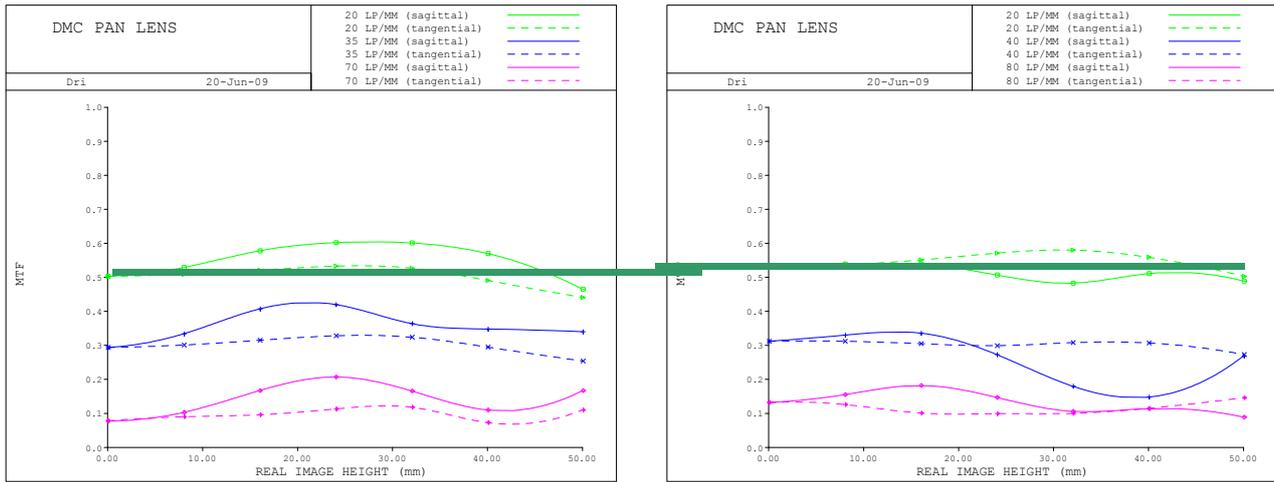
Fig. 12: MTF curves of the DMC Pan Lens at different flight heights indicating 5% MTF change at half the Nyquist frequency (green line) and 8000m height change.
