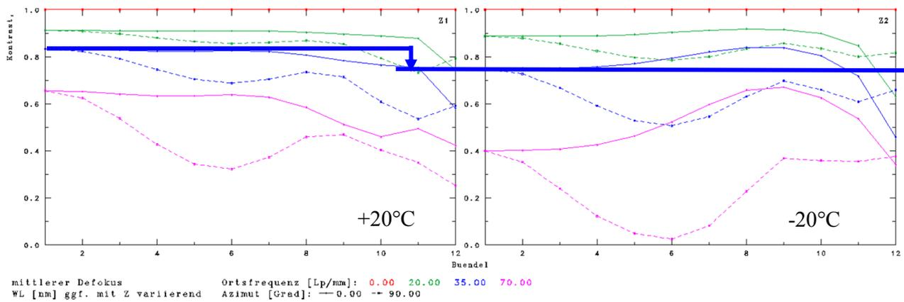
Fig. 10: MTF curves of the RMK-D Lens at different temperatures indicating 12% MTF decrease at half the Nyquist frequency and 40K temperature change.
