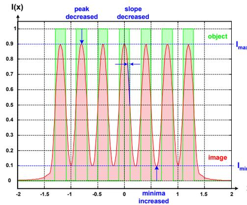
Fig. 3: Sketch of a grating image and reduction of contrast [6].
