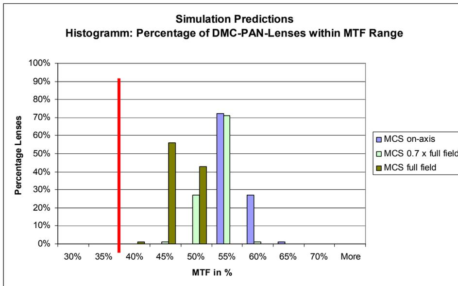
Fig. 15: Histogram simulated as-build MTF performance for DMC – PAN lens.
