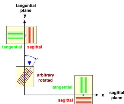
Fig. 4a: Orientation of the structure in the object.
