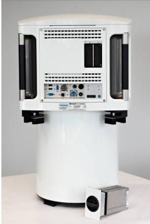
The storage system of the UltraCamL/Lp (left image) consists of an in flight exchangeable data unit with solid state devices. Each data unit has 1 TB of memory which lasts for around 2500 uncompressed images. The in flight exchange can be done in less than three minutes which leads to an “unlimited” storage in the aircraft due to multiple data units. So, there is no mission restriction due to the storage system of the camera.
