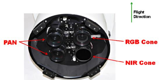
The RGB cone acquires the color information to color the pixels of the PAN image by the well know pan-sharpening methodology with a ratio of 1:2. The NIR cone collects NIR imagery with the same resolution than the RGB cone to support classification work. The PAN cones are lined up in flight direction and utilize the syntopic exposure for parallax free imagery, invented and patented by Vexcel for its large format cameras UltraCamD, X and Xp.
