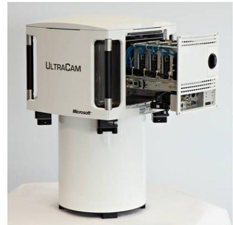
The UltraCamL/Lp also introduces a new service concept to the camera market. The computing subsystem (right image) is fully integrated into the camera head and very easy to access by a pull-out rack for service and maintenance. This reduces down-time in case of a service or maintenance.
