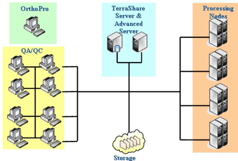
Figure 4. OrthoPro Distributed System
