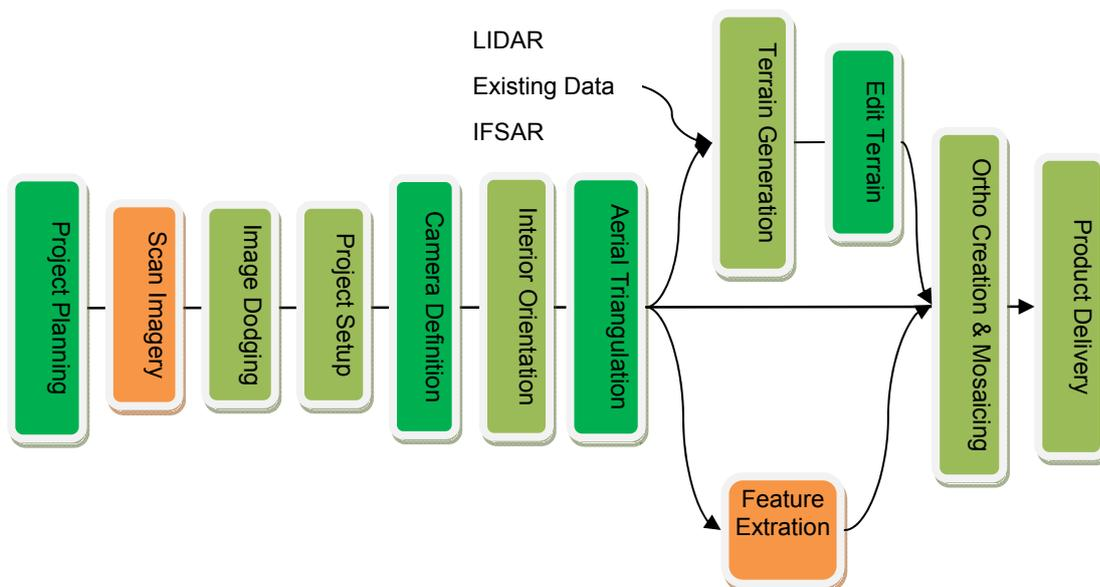
Fig. 1: Traditional Photogrammetric Workflow
