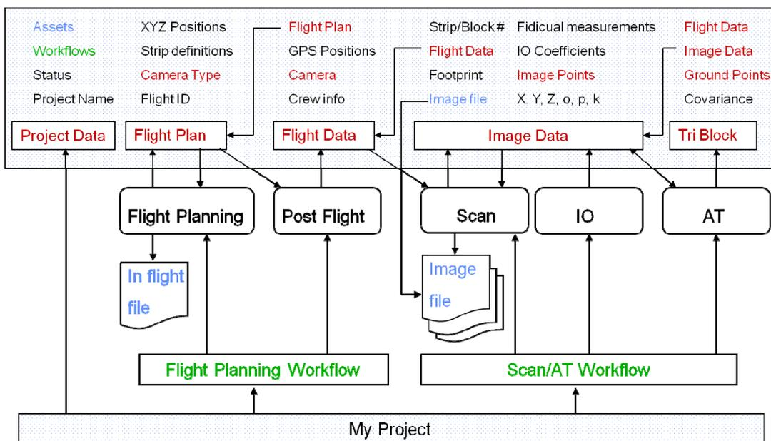
Fig. 5: Photogrammetric Data Model
