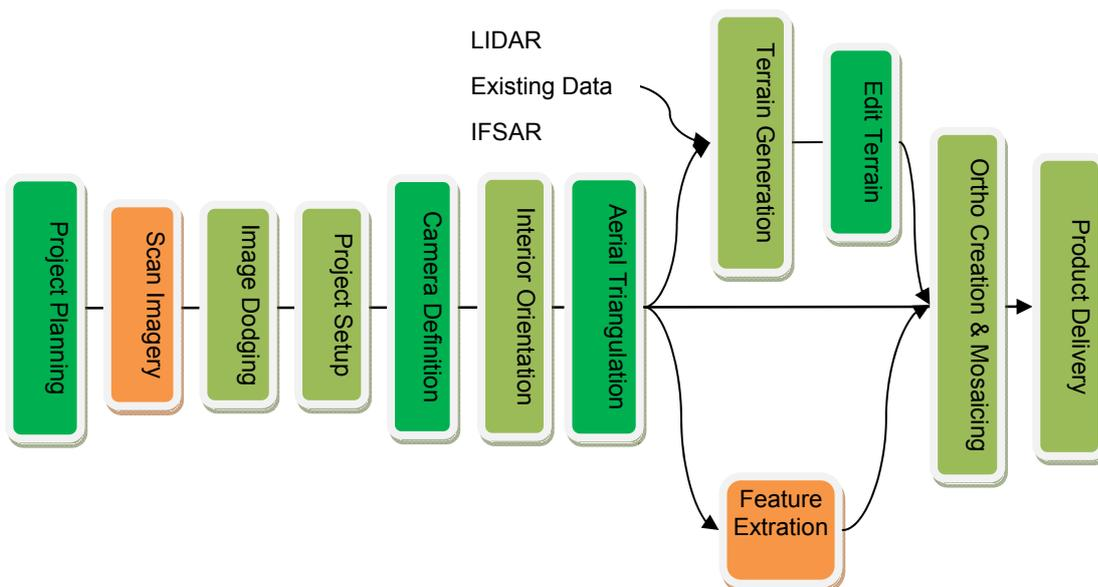
Fig. 1: Traditional Photogrammetric Workflow
