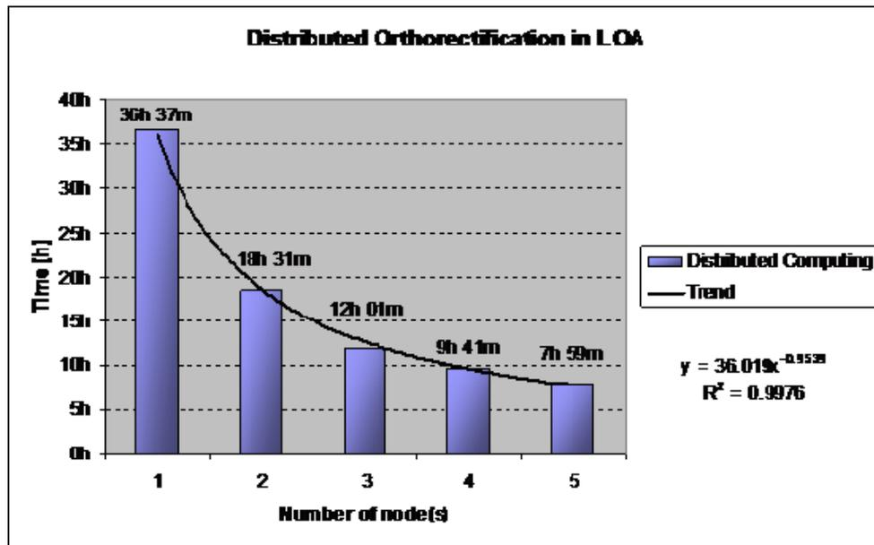
Fig. 4: Orthorectification time in hours and minutes for 858 images
