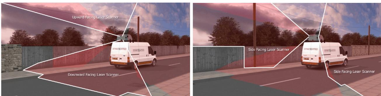
Figure 2: Field of view of the single laser scanners.
