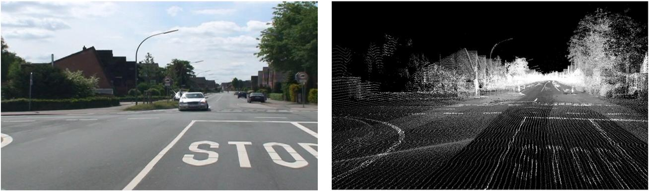
Figure 4: Street scene captured with video camera and the same scene in the lidar point cloud.
