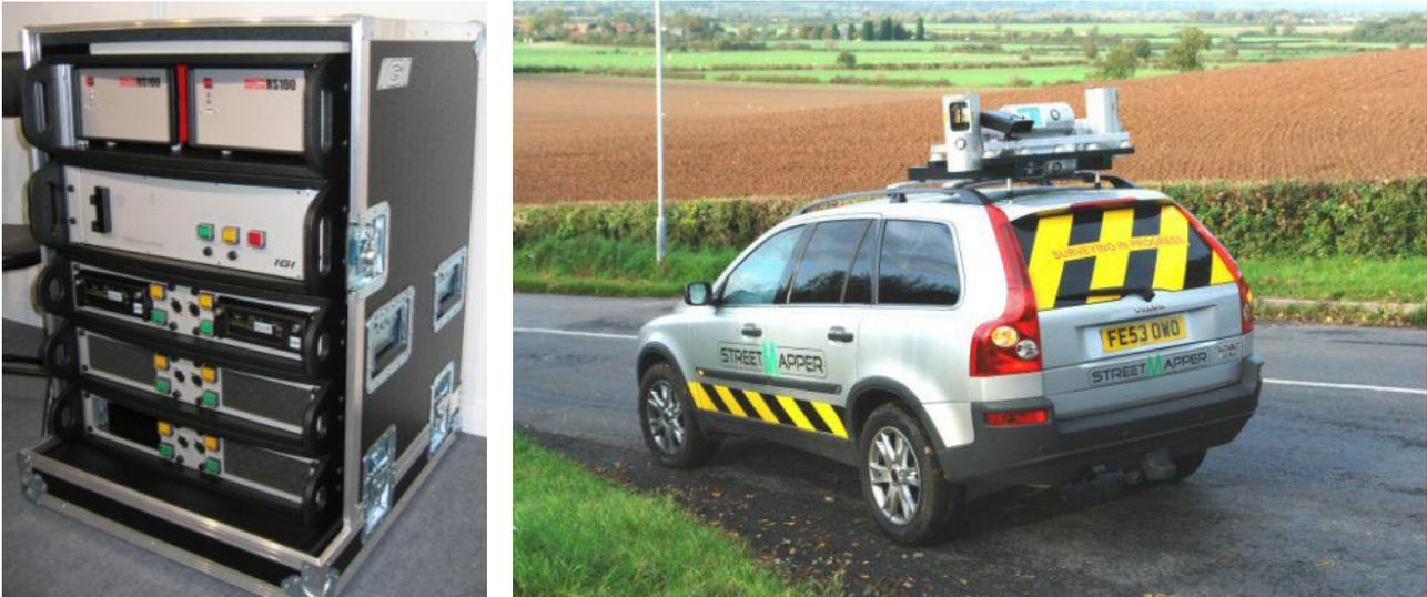
Figure 6: Left: StreetMapper electronic rack. Right: The sensor platform mounted on a vehicle.
