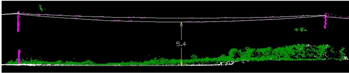
Figure 12: Measurement of the minimum vertical distance.
