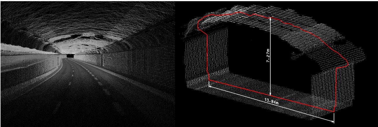
Figure 8: Measurement of a tunnel profile.
