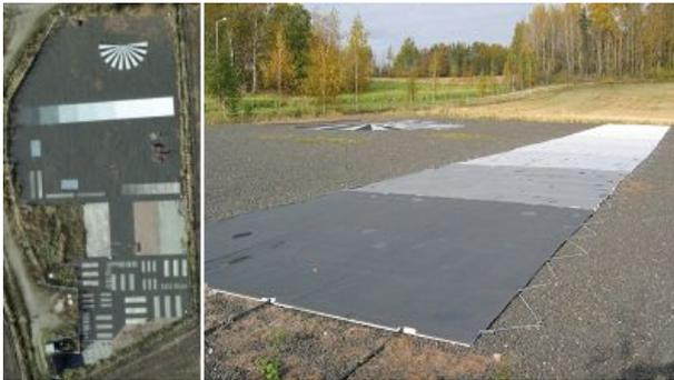
Fig 4. Left: The Sjökulla image quality test field. Right: The reflectance reference targets (8-step gray scale).
