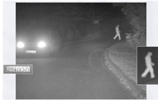
Fig. 8: Night scene illuminated with (NIR) high beam.
