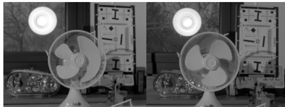
Fig. 5: Image distortion with high speed moving objects: HDRC sensor with rolling shutter readout (left image) and with a global shutter (right image).
