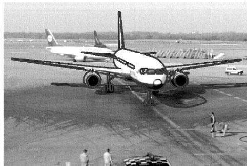
Fig. 9: Camera guided aircraft docking system using a HDRC® camera (courtesy: GEVITEC).
