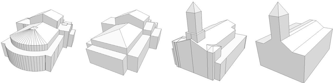
Fig. 9: 3D building models in their original (left) and generalised (right) shape.
