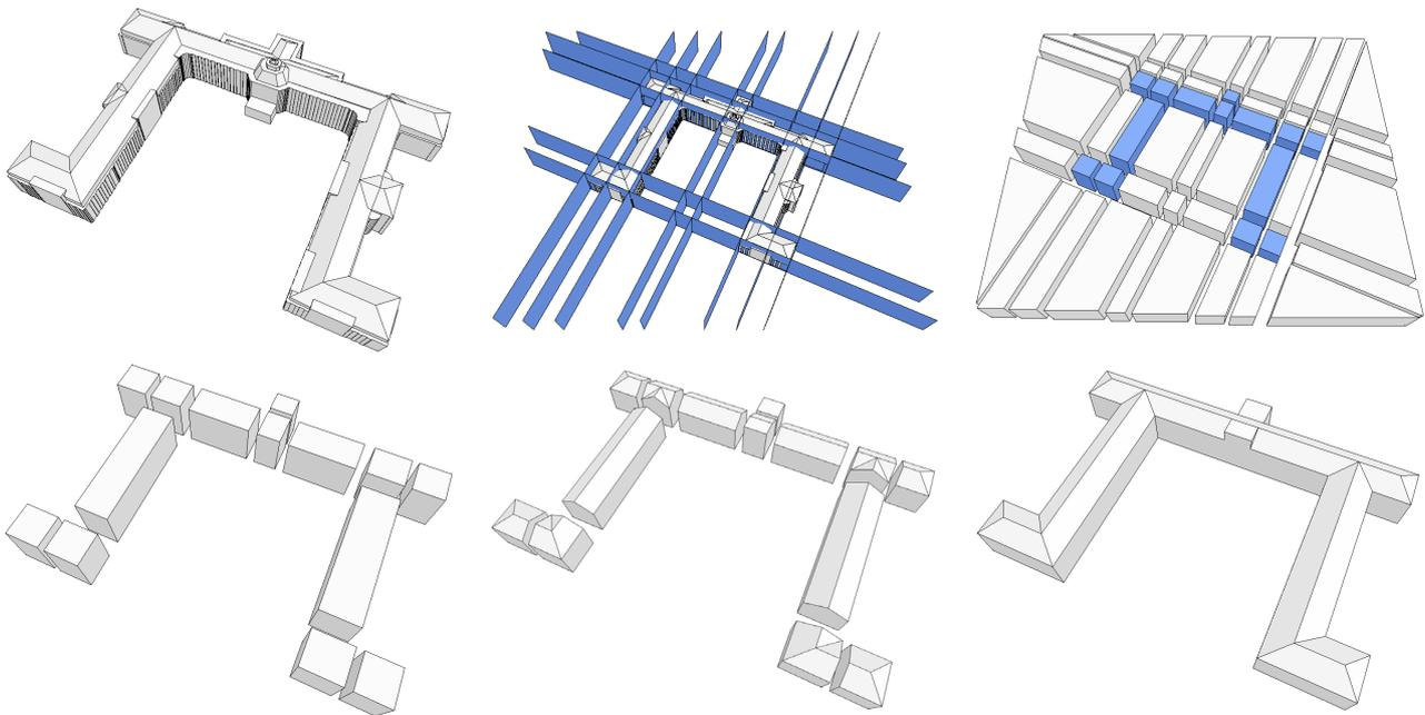
Fig. 5: Original 3D building model (top left) and the five generalisation steps.
