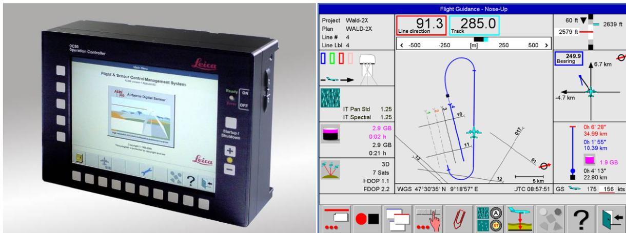
Figure 9. FCMS (Flight & Sensor Control Management System) shows the Pilot and Operator Controller OC50 for FCMS and Flight Guidance screen.
