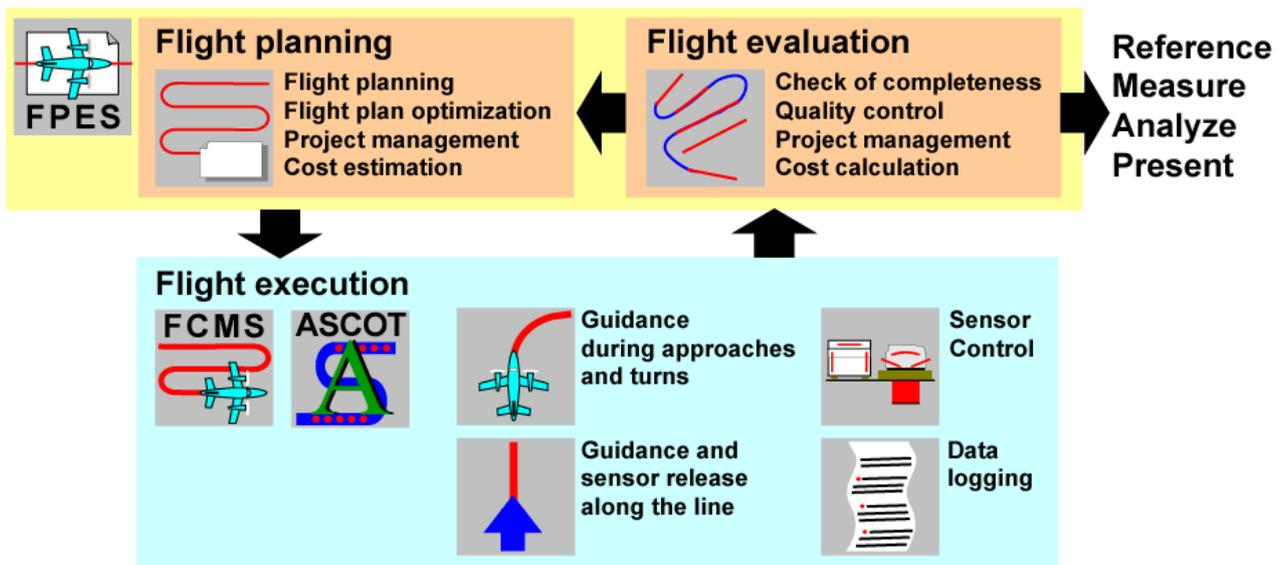
Figure 8. FPES Flight Planning & Evaluation System functional diagram.
