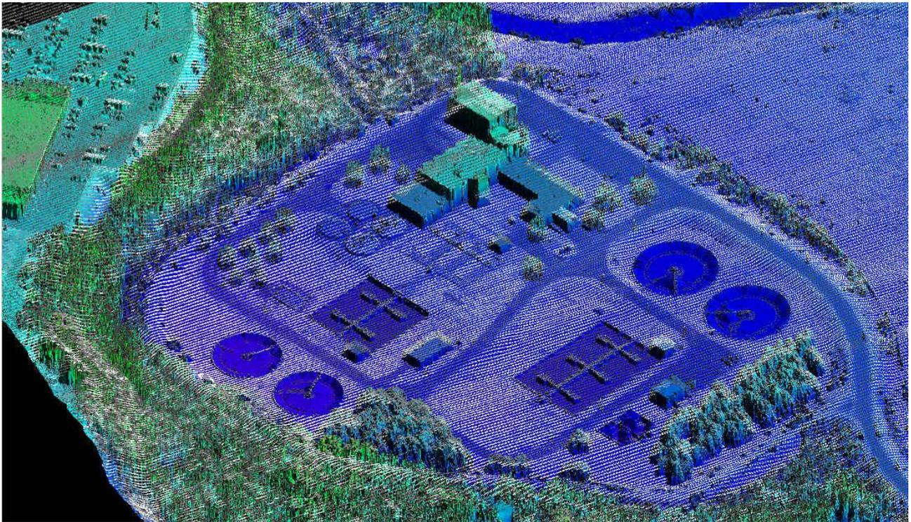
Figure 5. ALS50-II Airborne Laser Scanner sample image acquired at 1250m AGL at 150 kHz pulse rate using MPiA technology.
