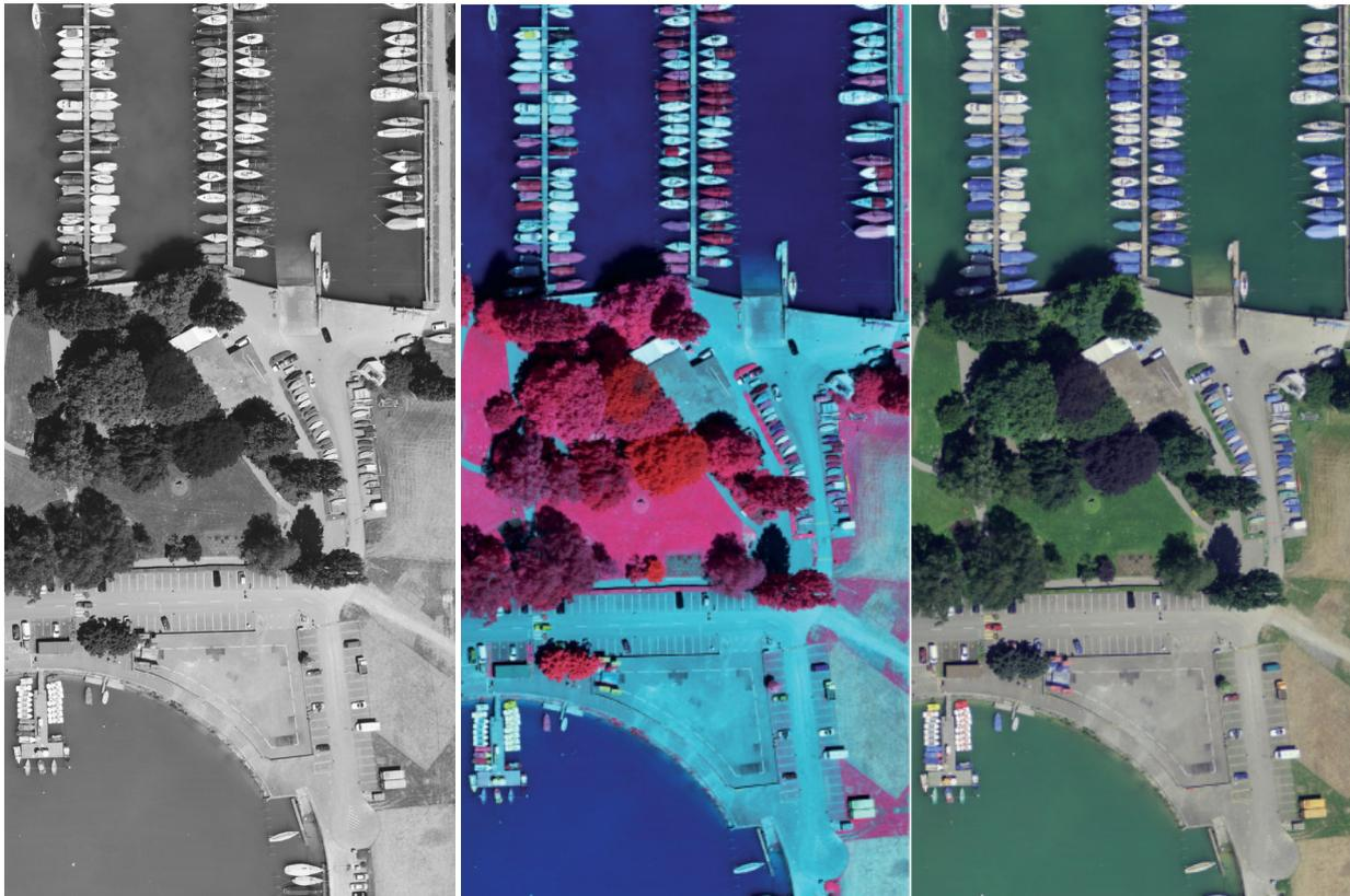
Figure 2. ADS40/SH52 co-registered Pan, RGB and CIR images. Romanshorn, GSD=10cm, Flying height = 1000m.
