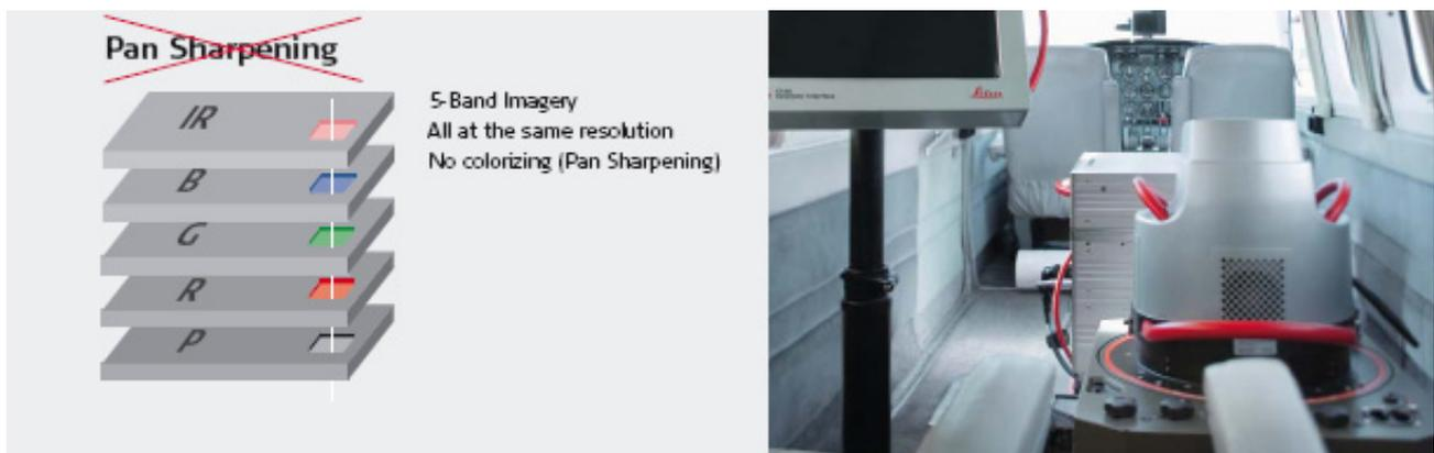
Figure 3. ADS40 2<sup>nd</sup> Generation Airborne Digital Sensor perfectly coregistered band concept and in-aircraft configuration.
