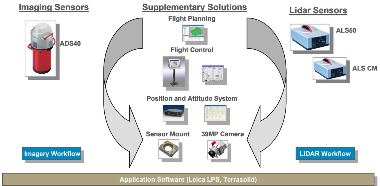
Figure 1. Leica Geosystems Airborne Sensors (ABS) family of products.
