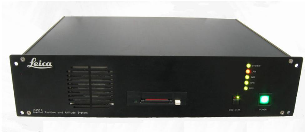
Figure 7. Leica IPAS10 GPS/IMU flight trajectory sensor unit standalone version.
