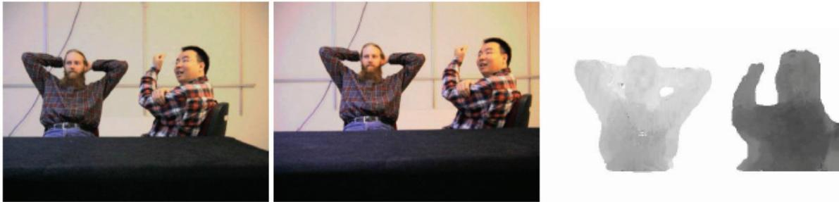
Fig. 12 Image pair from stereo video sequence (left) and depth map (right), determined in real-time; from YANG & POLLEFEYS (2003)
