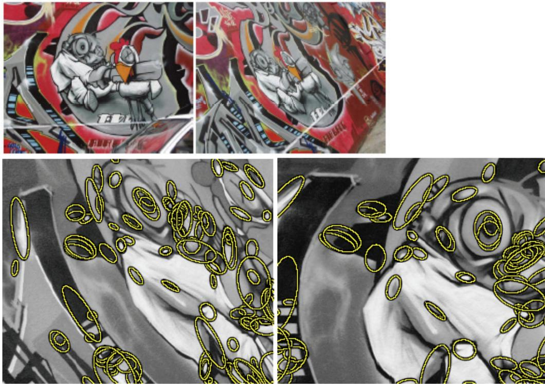
Fig. 5 Upper row: original image and distorted image. Lower row: affine invariant regions of a subsection (Harris corners). Total CPU-time on 800x640: 0.0143 s, on Pentium 4.2 GHz Linux PC, direction (adapted from MIKOŁAJCZYK ET AL. 2005)
