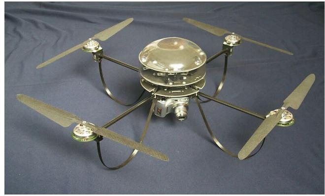
Figure 9: DigiFLY quadroheli with attached 7.2 MPixel digital camera
