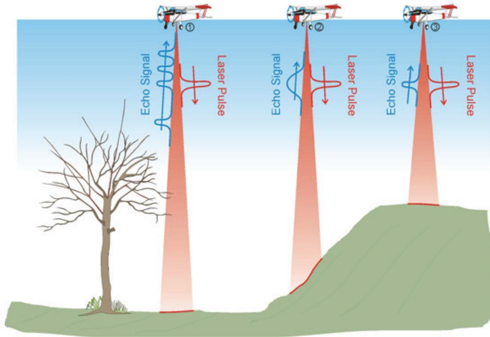
Figure 4: Waveform digitizing principle - Echo signals resulting from different targets [Riegler 2005]
