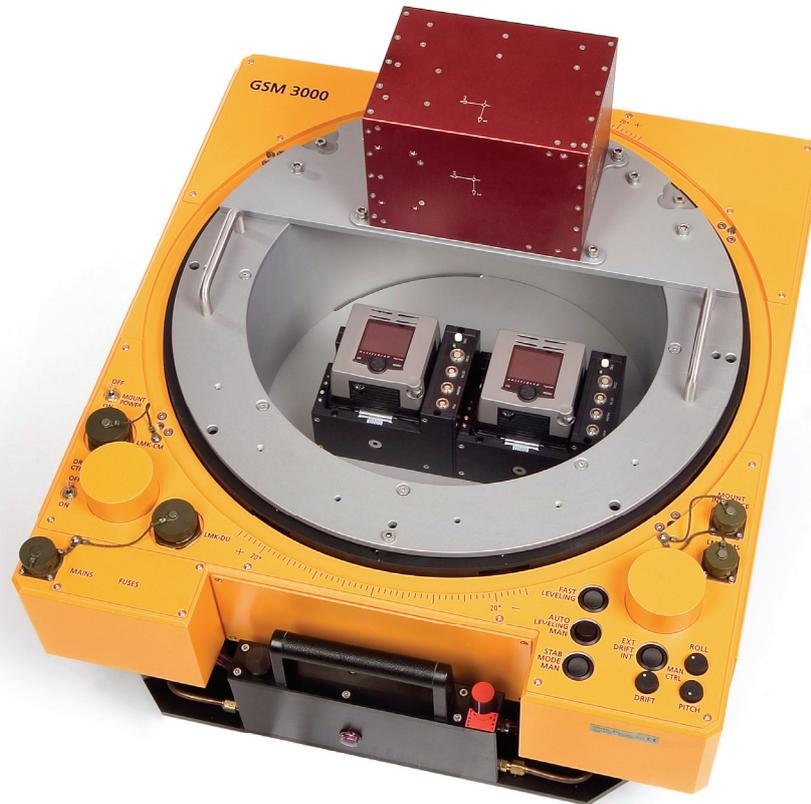
Figure 2: Two *DigiCAM* systems (RGB & CIR) mounted in a camera-pod to be operated in a GSM3000 mount
