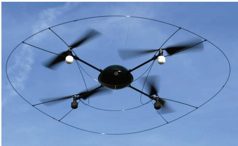
Figure 7: *DigiFLY*, a battery powered helicopter of the type quadroheli
