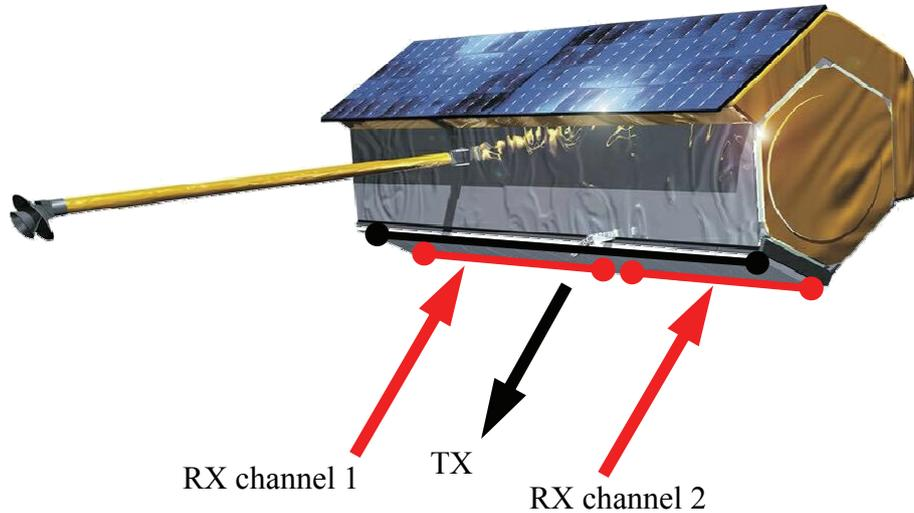
Figure 6: The radar antenna of TerraSAR-X electrically split in two halves on receive
