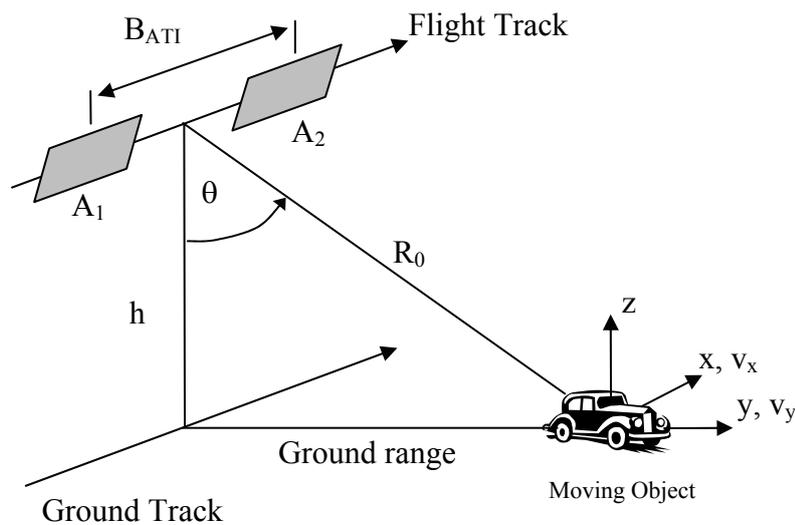
Figure 5: Principle of along-track interferometry (ATI)
