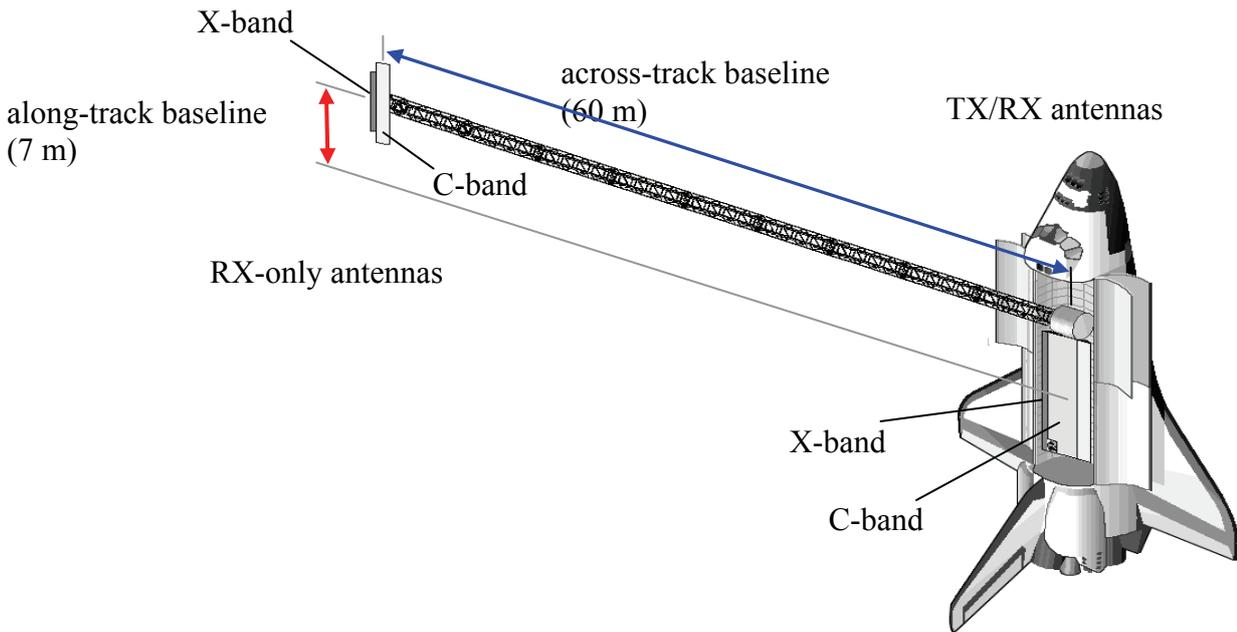
Figure 7: The interferometric configuration of SRTM. The displacement of the mast mounting away from the phase centers of the TX/RX antennas creates an along-track baseline component of 7 m.
